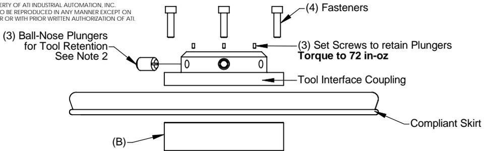
Dust Cover Assembly Exploded View
