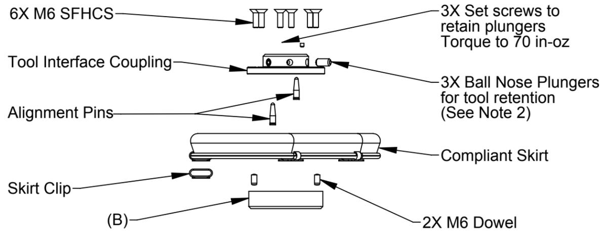
**Dust Cover Assembly Exploded View**
