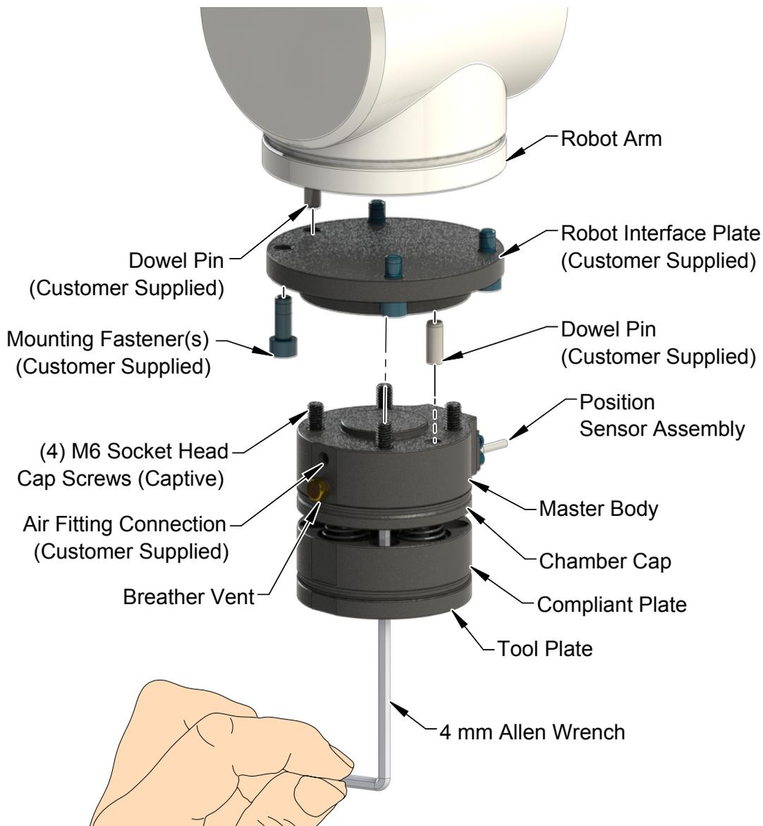
5. Once the compensator is attached to the robot, the customer tooling or tool interface plate can be attached. Refer to [Figure 4.2](#).
