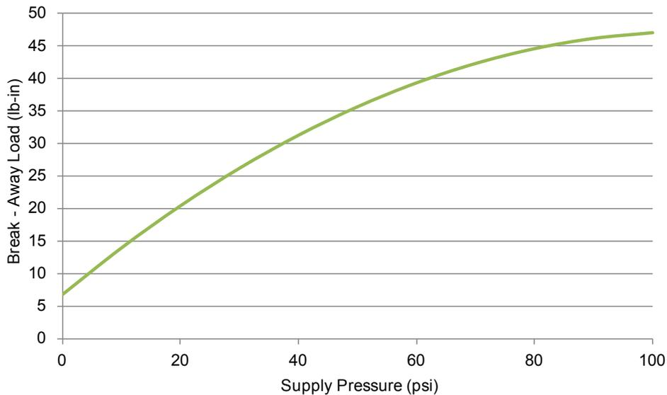
In [Figure 3.7](#), the Z Moment break-away is defined as 0.1° torsional displacement.
