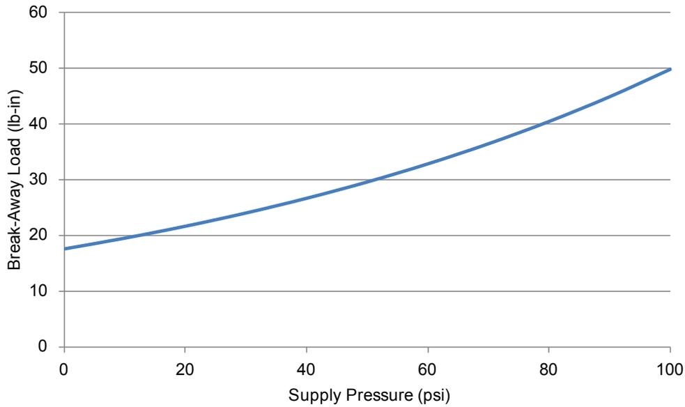
In some cases, it may be useful to estimate loads and deflections BEYOND the break-away point. Refer to [Figure 3.8](#) for an estimate of the expected angular deflection (rotation about the X or Y axis) as a function of the applied moment X-Y load and the air pressure supplied. For more information, refer to [Section 10—Drawings](#). Refer to [Figure 3.8](#) for calculating static X-Y moment, which is a function of the payload weight and distance to the payload center of gravity.
