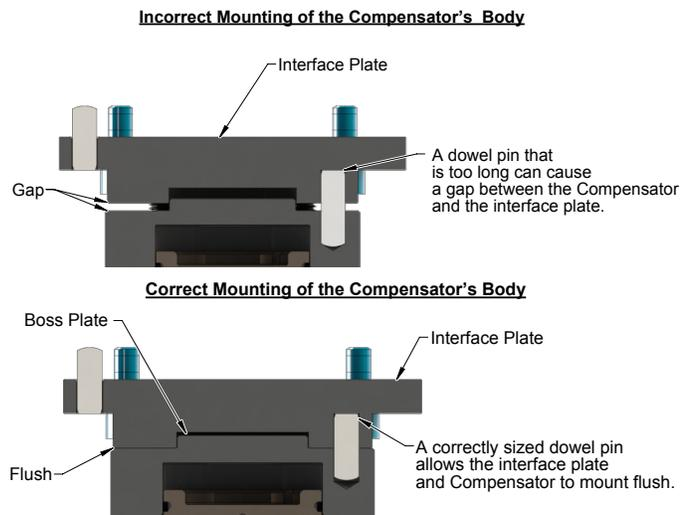
If the customer chooses to design and build a robot interface plate, consider the following points:
