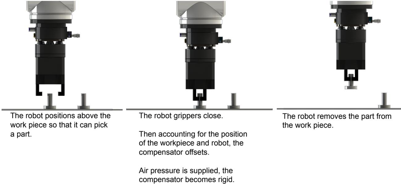
**Figure 5.4—Pick Part Operation Compressive, Angular and Torsional Direction**
