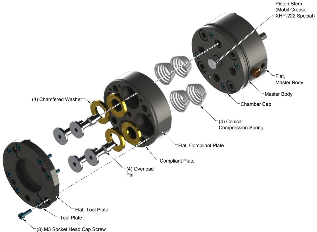
8. Apply XHP-222 special grease to the piston stem.
