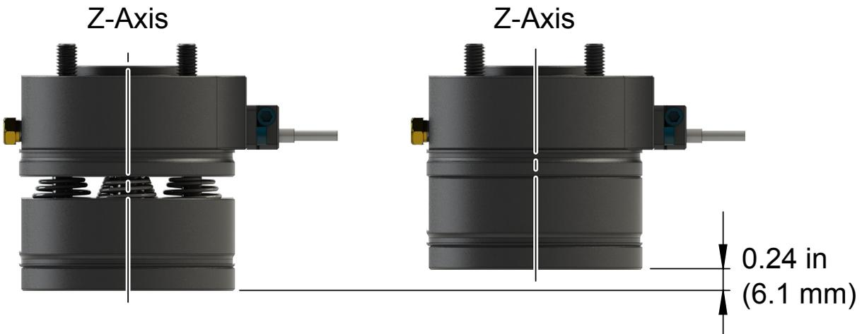
During torsional compliance, the compliant plate rotates about the Z axis, relative to the master body (see [Figure 3.3](#)). A small amount of compression along the Z axis due to unseating of the conical reset surfaces. Refer to [Section 9—Specifications](#).
