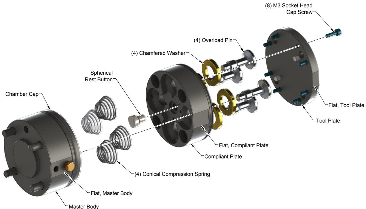
9. Press the new spherical rest button into the compliant plate.
