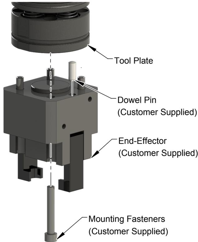
6. Secure the customer tooling or tool interface plate to the tool plate of the compensator using the customer supplied (4) M6 fasteners. Refer to [Table 4.1](#) for proper torque and Loctite specifications. Refer to [Section 10—Drawings](#) for mounting details.
