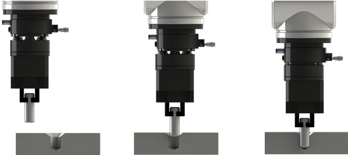
Robot moves to an insertion position above the work piece.
