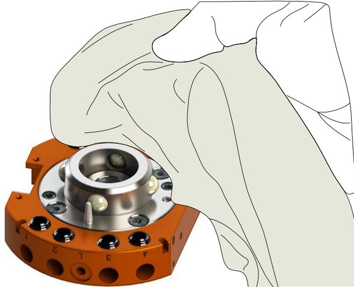
5. Use a clean rag to thoroughly remove any lubricant and debris from the inner surface of the male coupling and cam.
