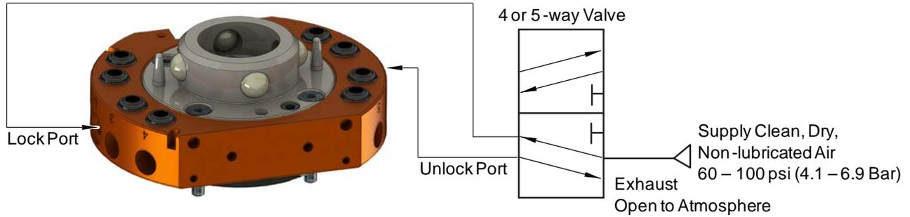
**Figure 3.21—QC-27 Lock and Unlock Pneumatic Connections**
