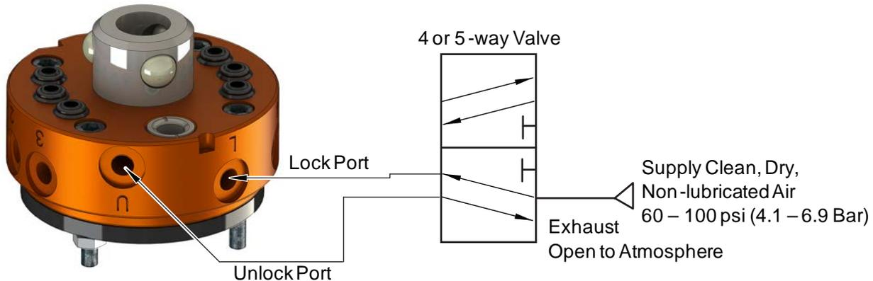
**Figure 3.20—QC-20 and QC-21 Lock and Unlock Pneumatic Connections**
