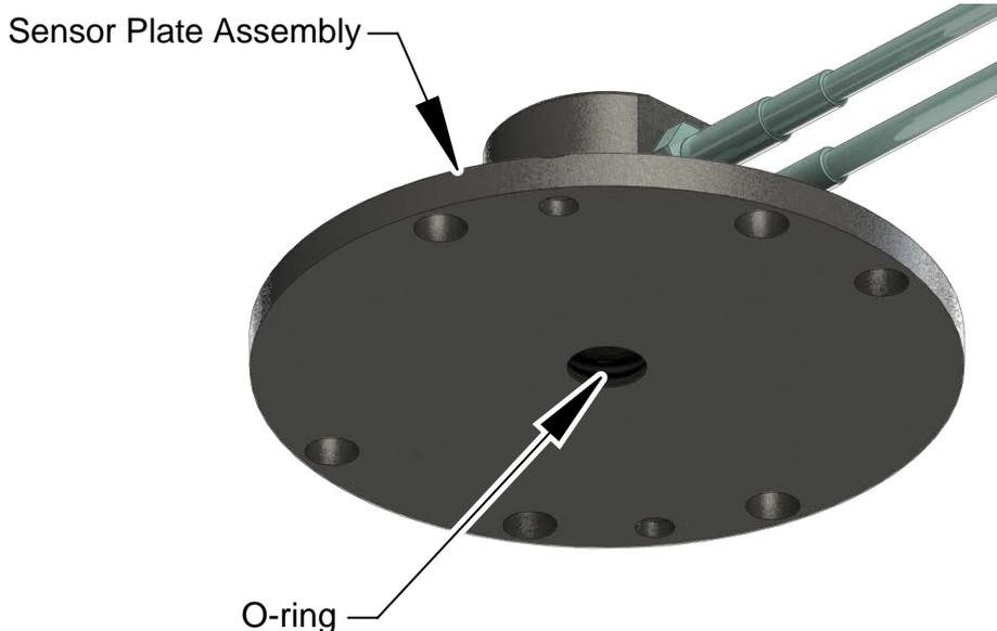
8. Press the detection shaft into the sensor plate assembly; push the shaft all the way through until it stops.
