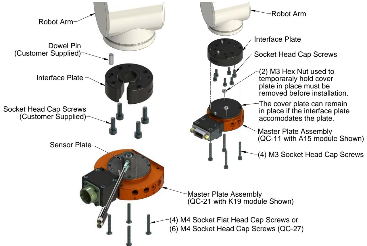
5. If equipped, connect the Lock and Unlock sensor cables.
