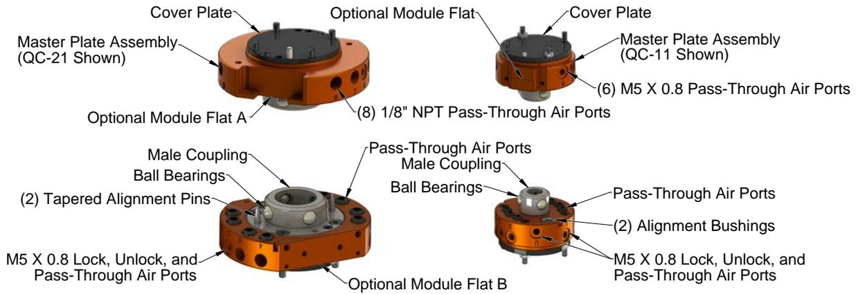
The air ports provide Lock and Unlock air for the locking mechanism and pass-through air for the end of arm tooling. An adapter plate assembly provides a standoff for the air ports and a mounting pattern to attach to the robot arm.
