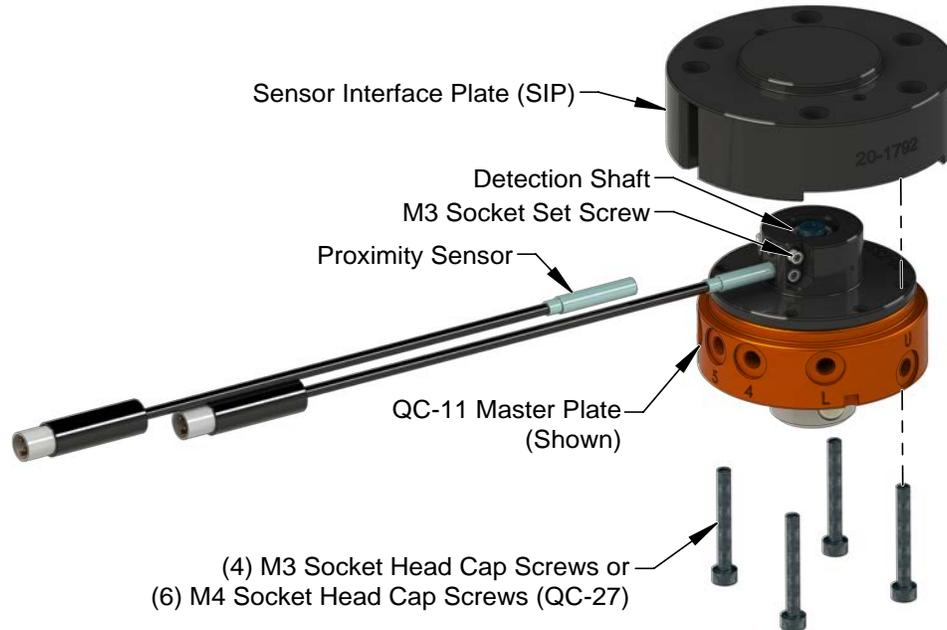
9. From a top-down view of the sensor plate assembly, verify the detection shaft does not touch the Lock and Unlock sensors. If the sensors touch the shaft, adjust the sensor position.
