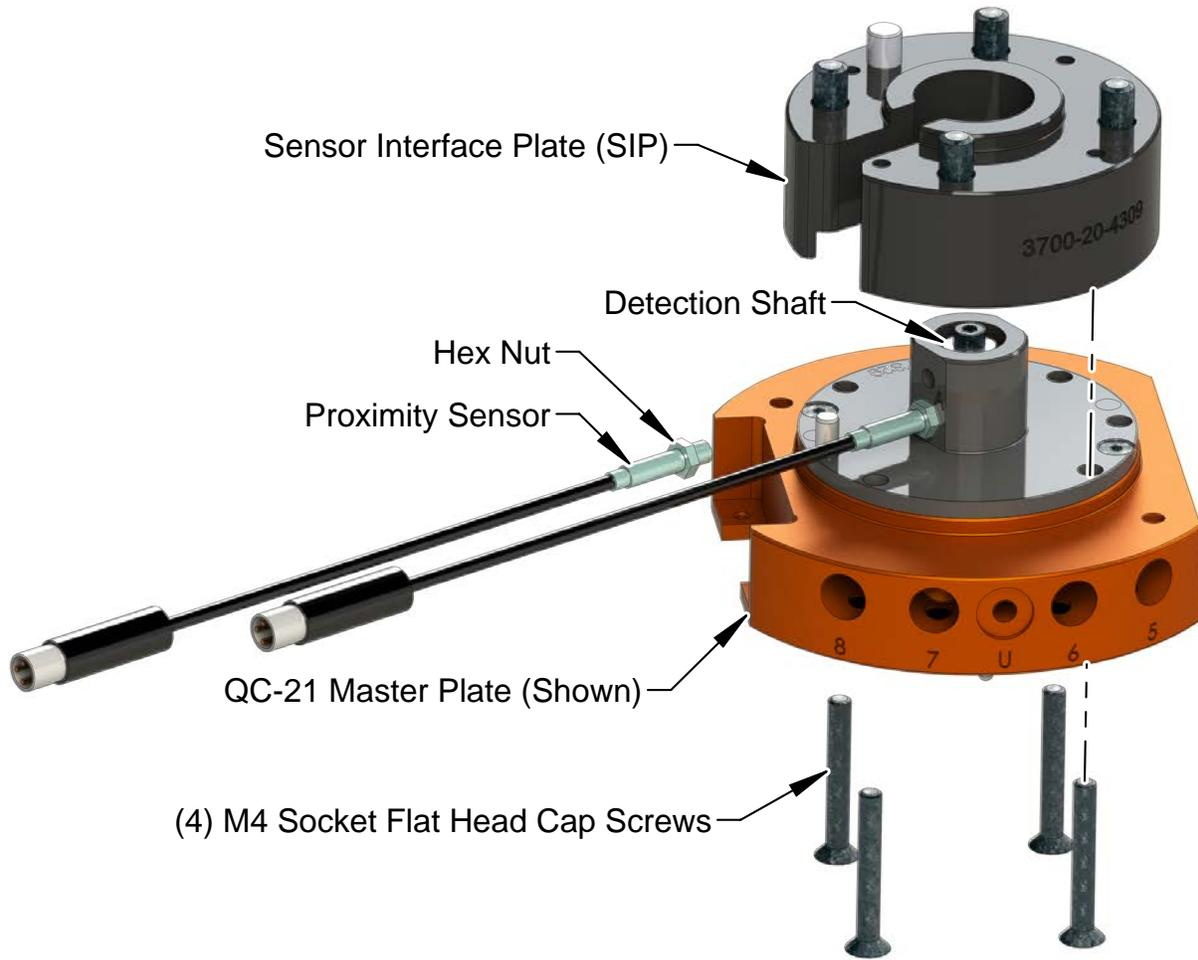
8. On the new sensor, back the sensor hex nut to the cable end of the sensor.
