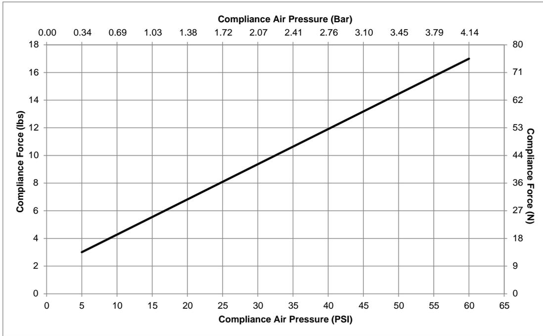
**Figure 2.4—Axial Compliance Force (Measured at the Tool Tip)**
