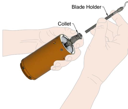
4. Adjust the blade holder to the desired height, confirm divots and ball lock are aligned.
