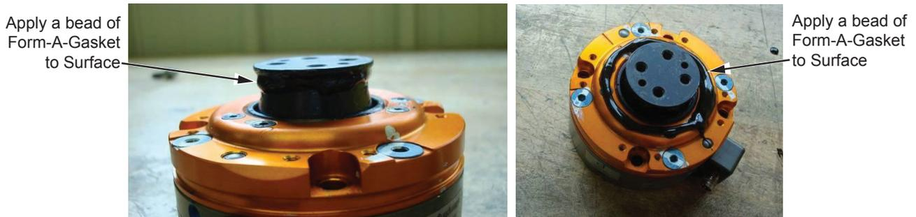
3. Install boot by stretching the center hole over the stem. Line up the screw holes and clearance slots with those in the cover plate.
