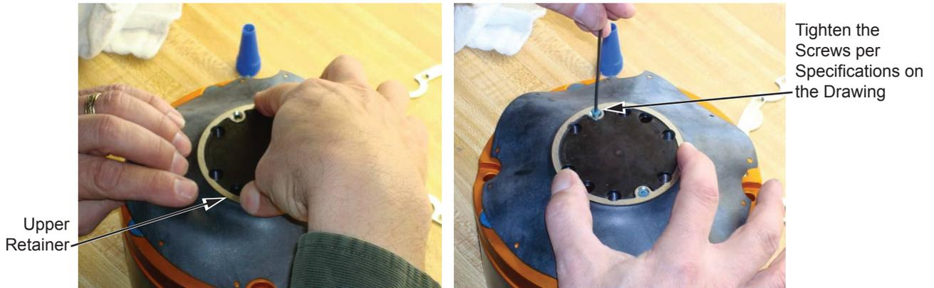
7. Place the lower retainer over the boot and cover plate. Thread the (12) flat head socket head cap screws into the tapped holes in the cover plate. Do this progressively to pull the boot down evenly. Tighten screws to 32 in-oz (0.23 Nm).
