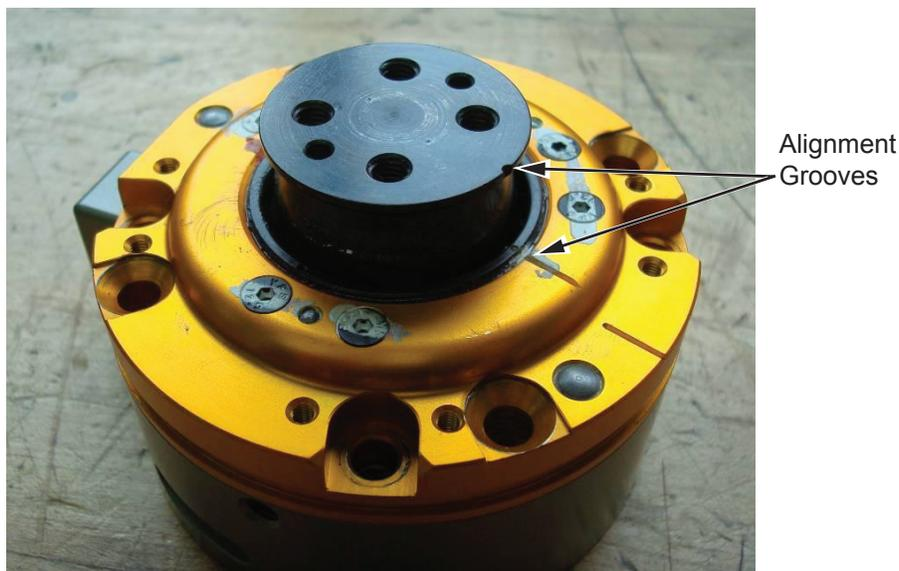
4. Place the stem and cover plate together onto the body. Make certain that the dowel pins in the cover plate are aligned with the holes in the body and that the alignment grooves in the cover plate and the stem are still aligned.
