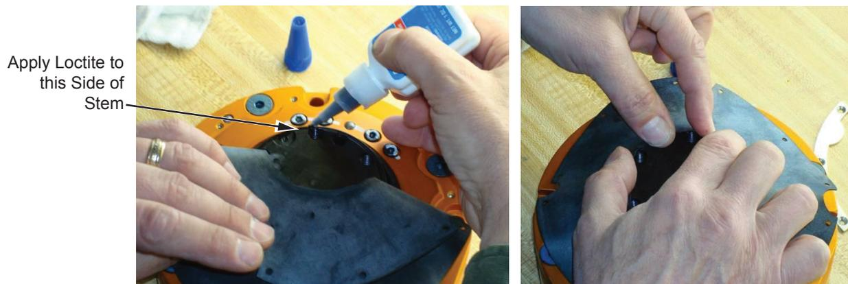
6. Place the upper retainer onto the stem. Thread the flat head socket head cap screws into the tapped holes in the stem. Tighten screws to 96 in-oz (0.68 Nm).
