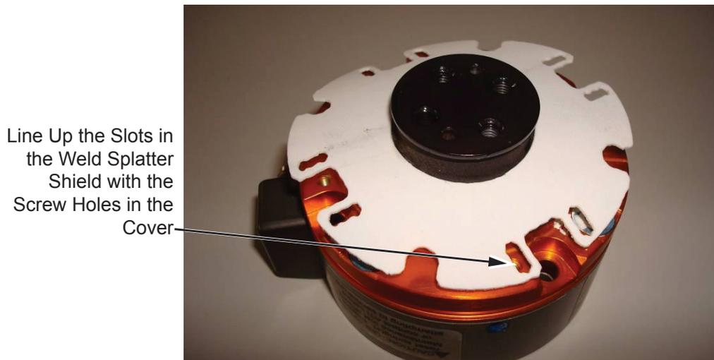
4. Insert the flat head socket head cap screws through the boot retainer and place the boot retainers onto the installed weld splatter shield. Screw them into the tapped holes in the cover plate.
