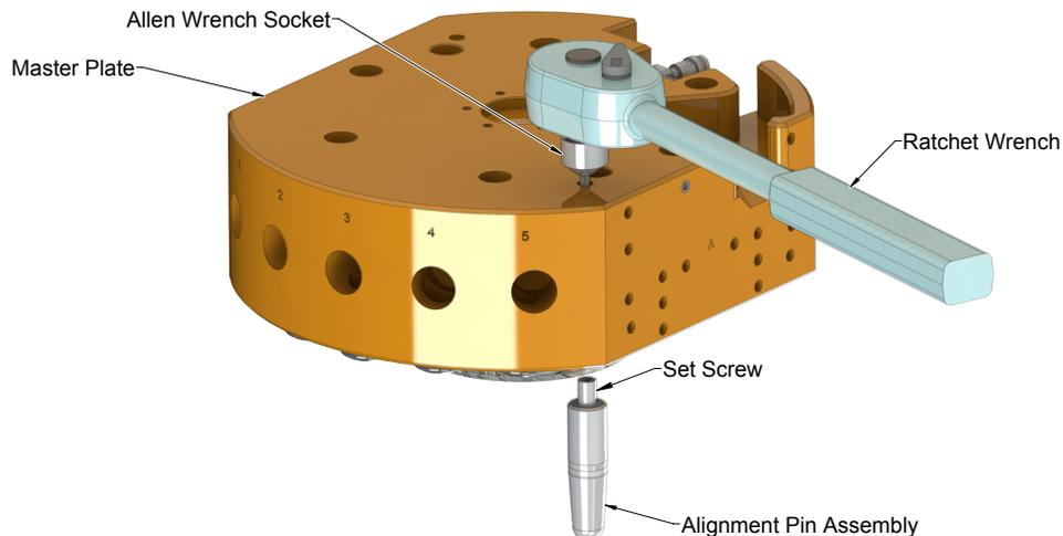
6. Once the alignment pin has been removed, verify that the assembly (pin and set screw) are intact. If the set screw portion of the assembly did not come out, it will be necessary to remove it separately using the access hole in the back plate of the Master plate.
