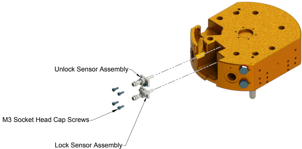
10. Insert the new Lock and/or Unlock sensor assembly into the Tool Changer body as shown in [Figure 5.7](#).
