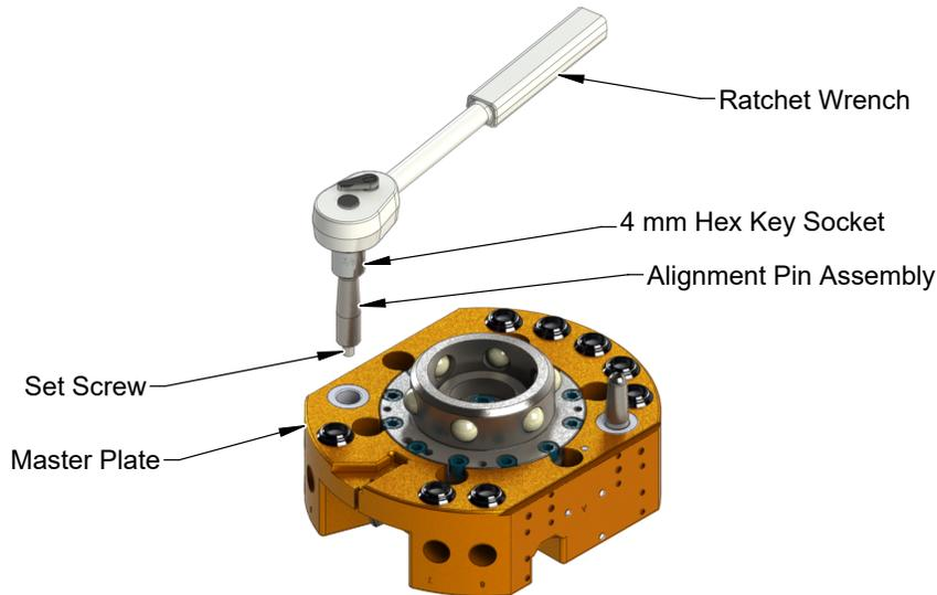
5. Another approach would be to use the access hole in the back side of the Master plate. If not already removed, remove the Master plate refer to [Section 2.3—Master Plate Removal](#). Use a 3 mm hex key to remove the alignment pin from the back side of the Master plate.
