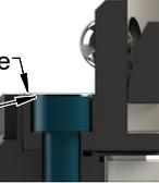
Head of Mounting Fastener Must Be Flush or Below Mating Surface. (Do Not Use Lock Washer under Head of Mounting Fastener.)
