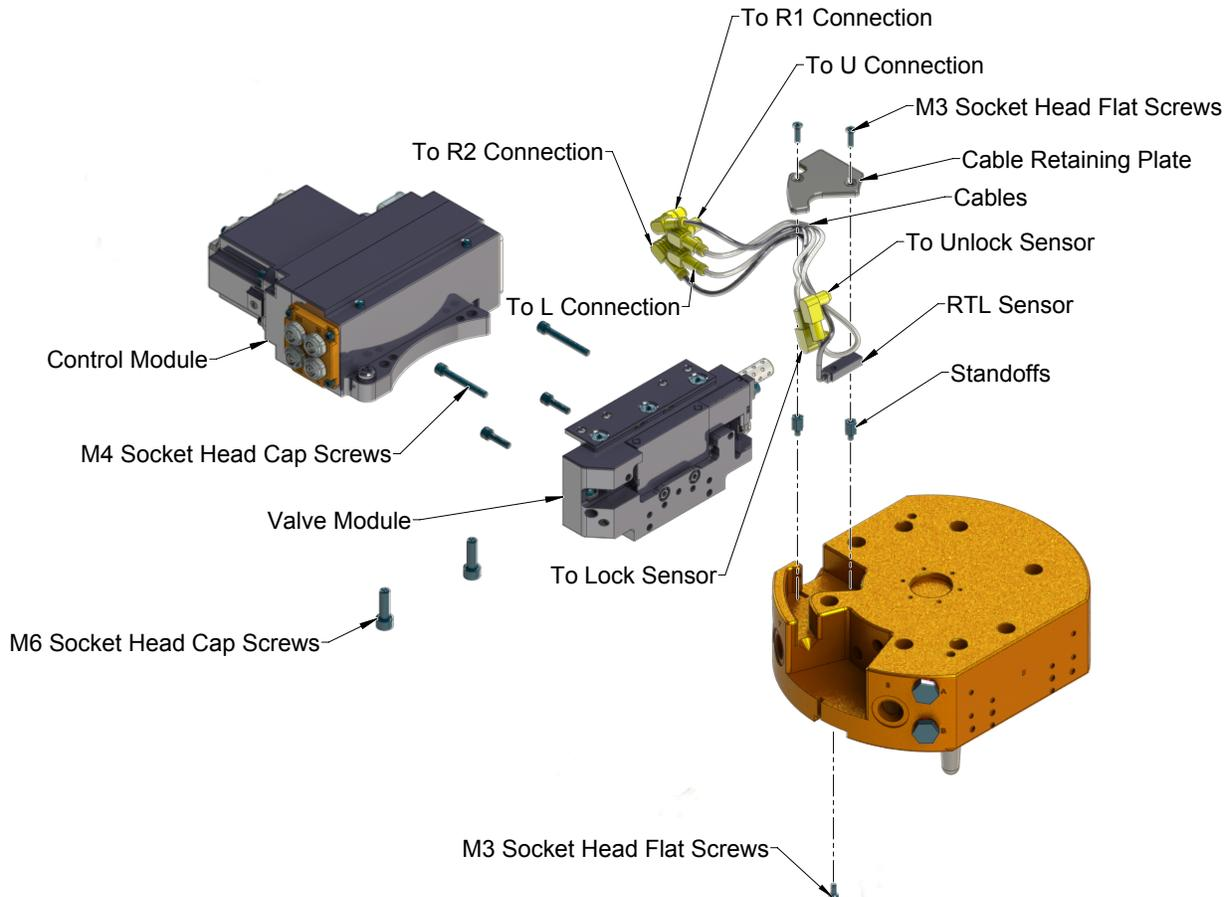
12. Install the new sensor cable into the cable channel of the Tool Changer body.
