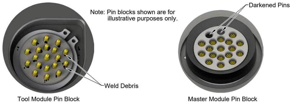
5. If debris or darkened pins are present, use a vacuum to remove the debris, and clean using a nylon brush (ATI part number 3690-0000064-60).
