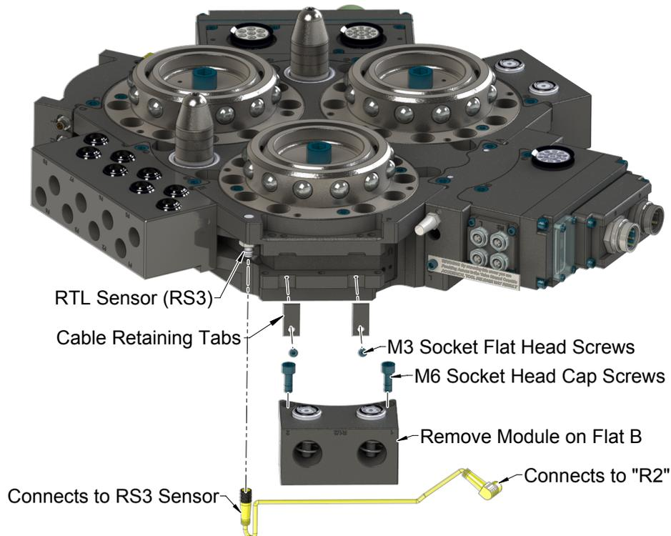
9. Connect the new cable connector to the control/signal module (R2) on Flat A.
