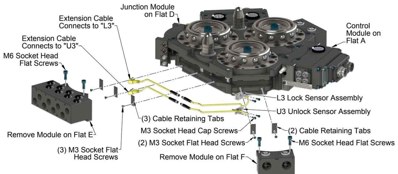
11. Pull the sensor assembly straight out from the Tool Changer body.
