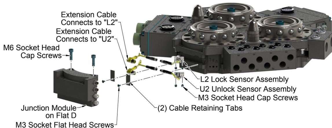
14. Insert the lock and/or unlock sensor assembly into the Tool Changer body as shown in [Figure 5.9](#). Ensure that new O-ring is in place before inserting sensor.
