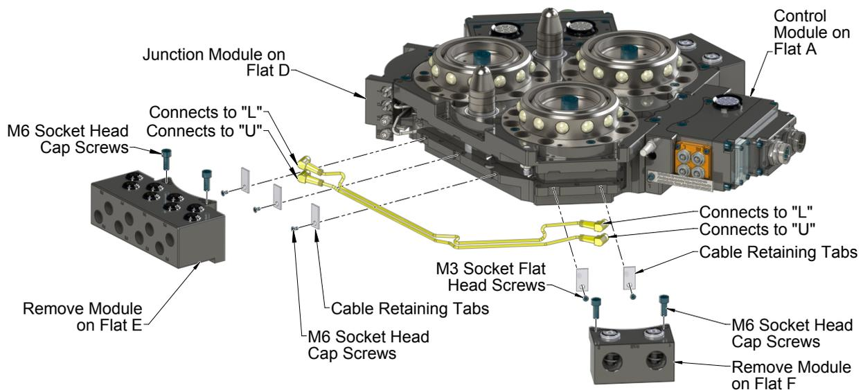
11. Route the new cable into the cable channel of the Tool Changer body.
