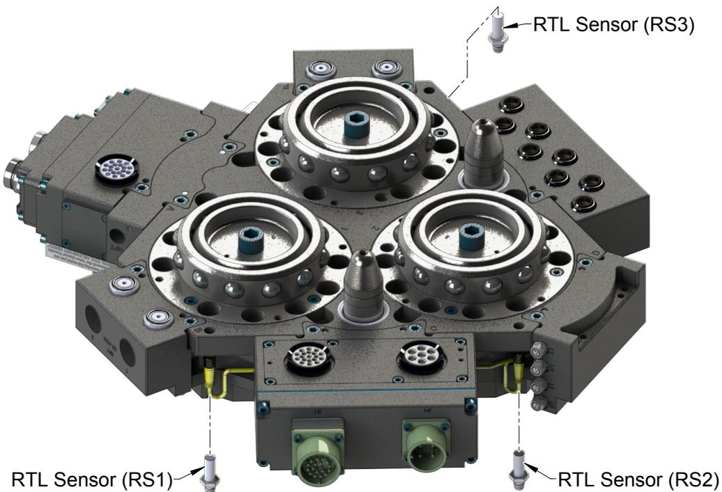
8. Apply Loctite 222 to and screw the new RTL sensor into the Tool Changer body until the face of the sensor is flush with the surrounding face of the Master body.
