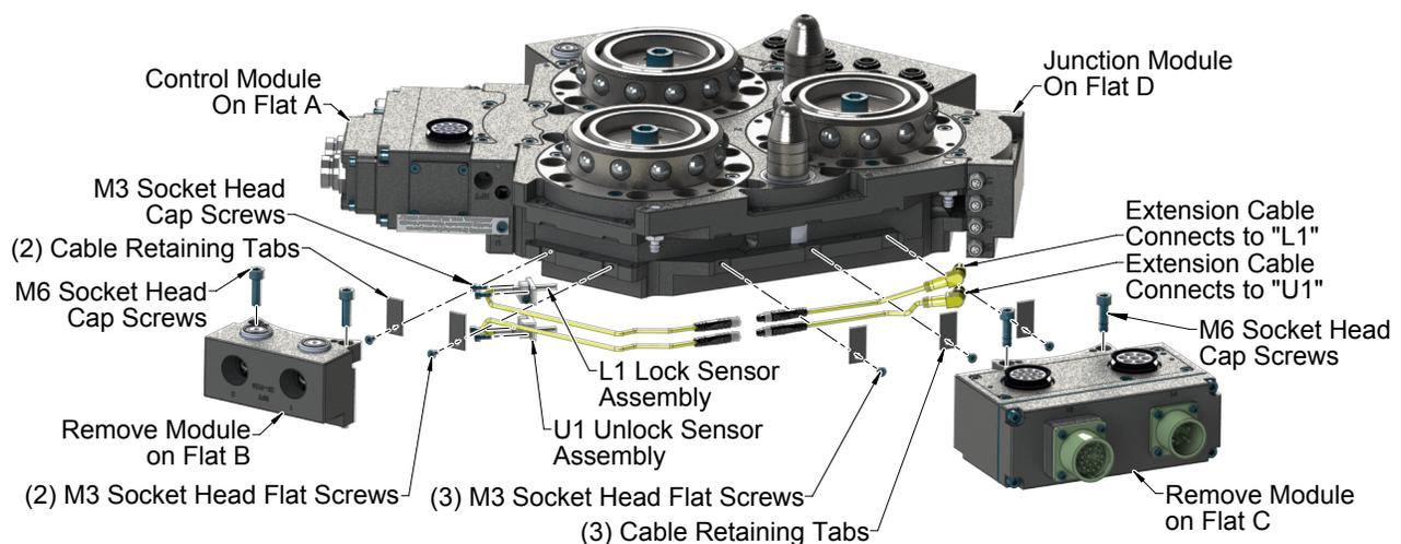
11. Pull the sensor assembly straight out from the Tool Changer body to remove the Lock and/or Unlock sensor assembly from the cable channel of the Tool Changer body. There is an O-ring around the cylinder barrel, ensure O-ring came off with old sensor before continuing. Discard the removed sensor assembly.
