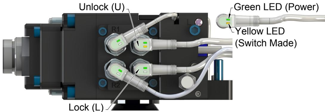
26. Confirm the operation of the lock sensor by locking the Tool Changer and then checking to see if the lock sensor cable LED is on.
