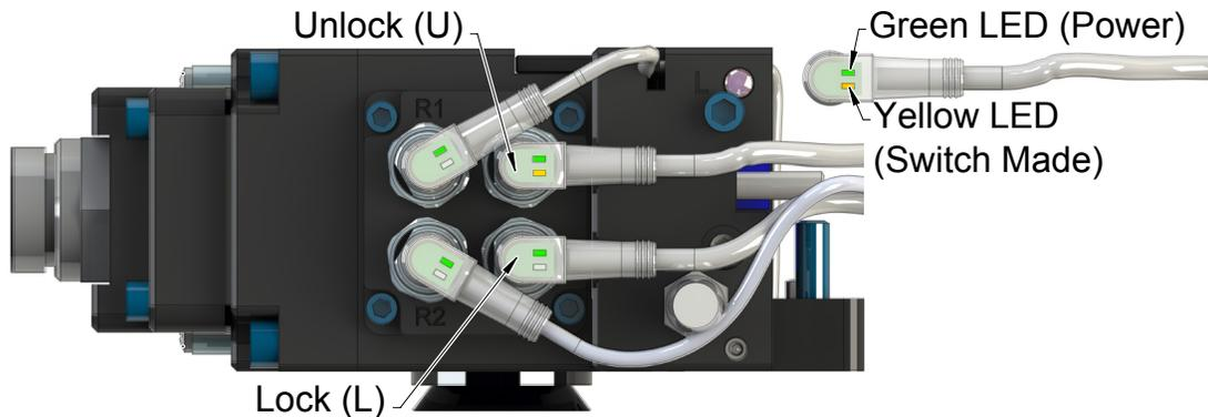
21. Confirm the operation of the Lock sensor by locking the Tool Changer and then checking to see if the lock sensor cable LED is on.
