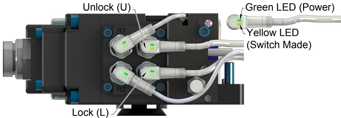
27. Confirm the operation of the lock sensor by locking the Tool Changer and then checking to see if the lock sensor cable LED is on.
