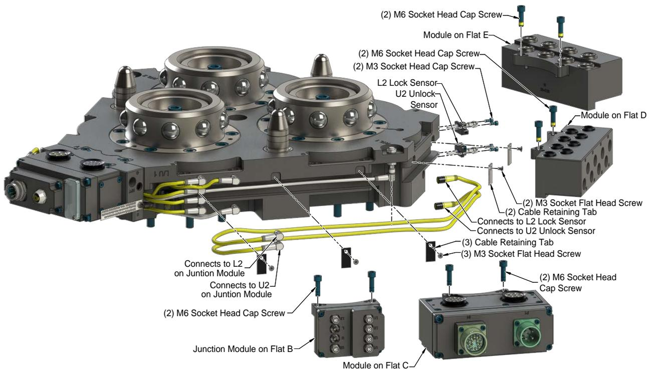
17. Reinstall all previously installed modules on Flat C and D.
