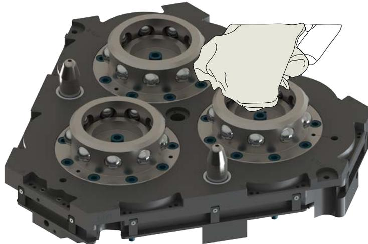
6. Check each ball bearing to make sure it moves freely in the male coupling. Additional cleaning may be necessary to free up any ball bearings that are sticking in place.
