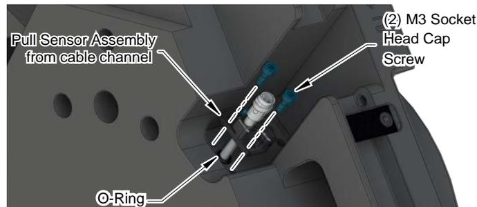
9. Install sensor assembly onto the Tool Changer body as shown in [Figure 5.4](#).
