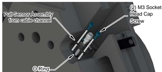
11. Install the new sensor assembly onto the Tool Changer body as shown in [Figure 5.10](#).
