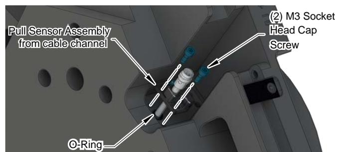
11. Install new sensor assembly onto the Tool Changer body as shown in [Figure 5.8](#).
