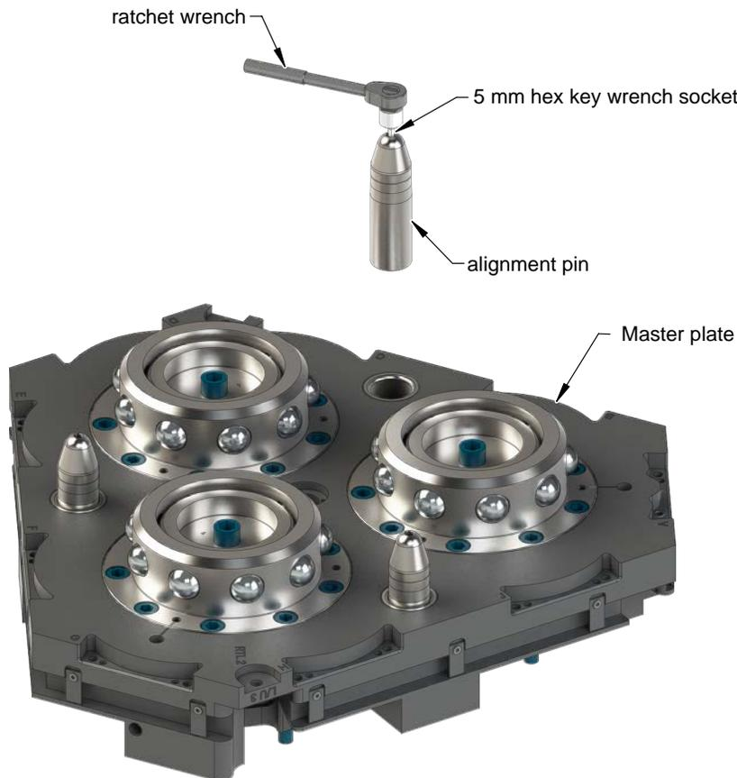
5. Apply Loctite 242 to the female threads of the alignment pin.
