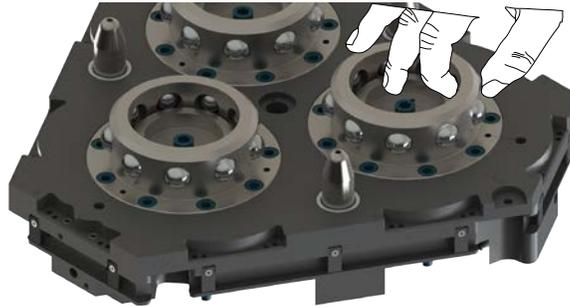
7. Apply a liberal coating of lubricant to the ball bearings, the male coupling (inside and out), and the alignment pins.
