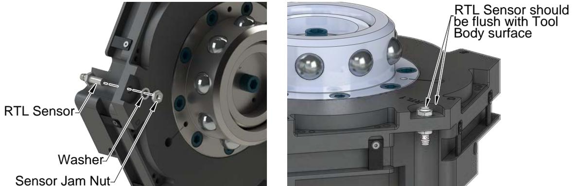
11. Connect the RTL sensor cable to the new sensor.
