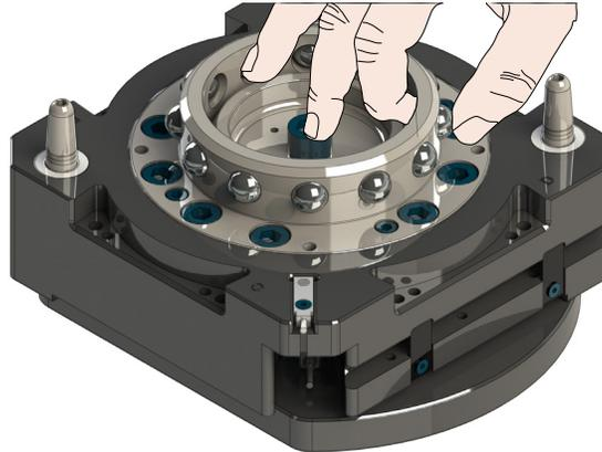
7. Apply a liberal coating of lubricant to the ball bearings, the male coupling (inside and out), and the alignment pins.
