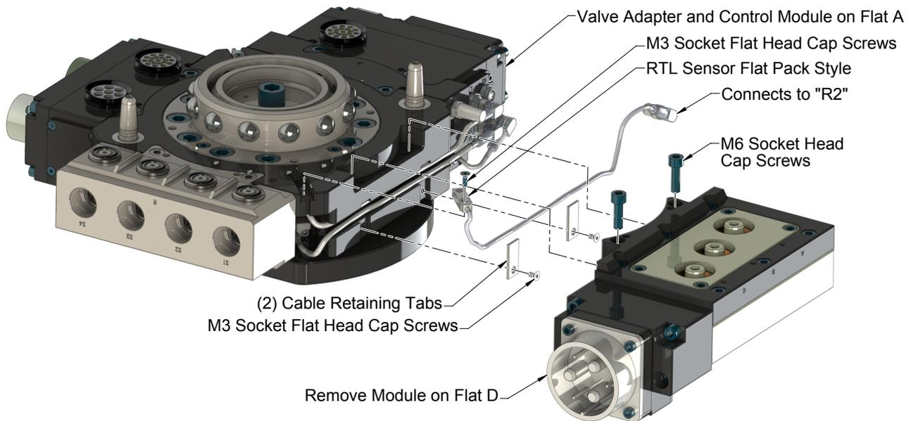
10. Install the new RTL sensor, routing the cable into the cable channel of the Tool Changer body.
