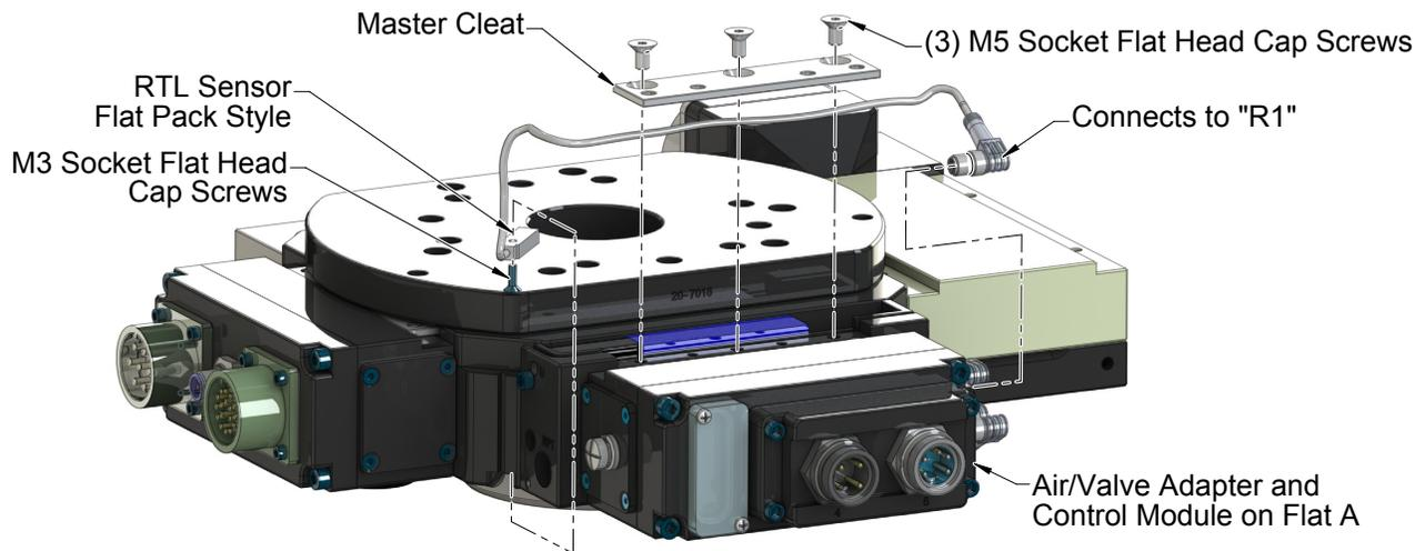
9. Install the new RTL sensor, routing the cable into the cable channel of the air/valve adapter.
