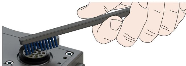
6. Inspect the Master and Tool pin blocks for stuck pins or pin block damage.
