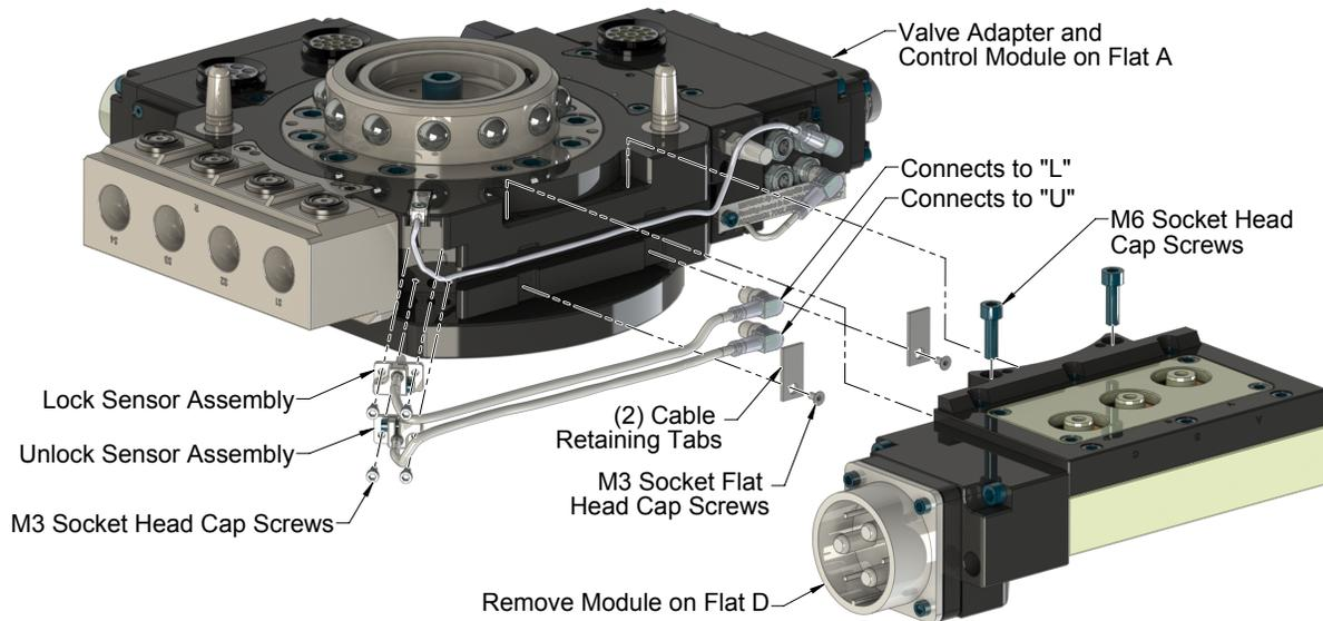
10. Install the new Lock and/or Unlock sensor assembly, routing the cable into the cable channel of the Tool Changer body.
