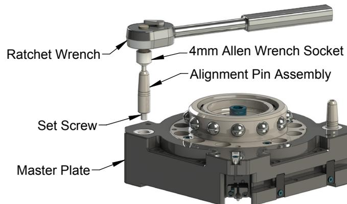
5. Another approach would be to use the access hole in the back side of the Master plate. If not already removed, remove the Master plate refer to [Section 2.3—Master Plate Removal](#).
