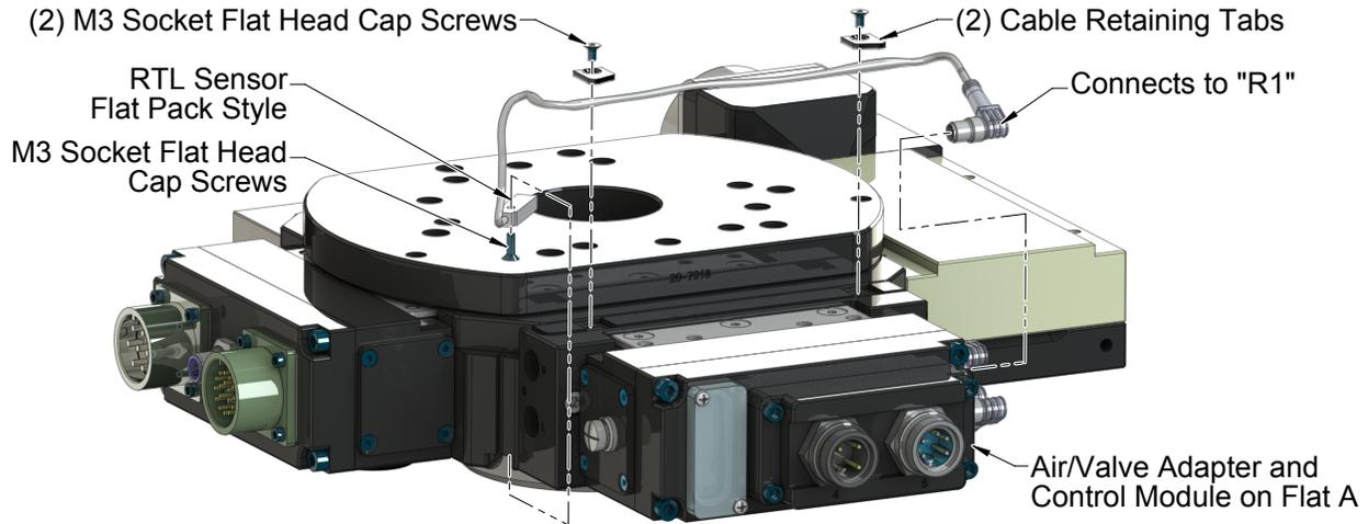
**Figure 5.7—RTL (R1) Sensor Assembly Replacement with Master Cleat**
