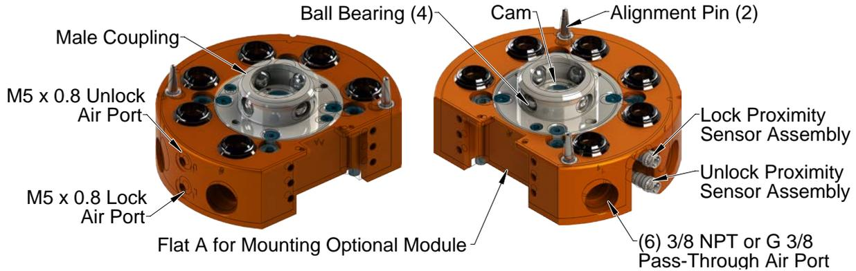
Tapered pins located on the Master plate mate with bushings in the Tool plate to ensure repeatable alignment during the coupling process. An extreme pressure grease is applied to the cam, male coupling, ball bearings, and pins to enhance performance and maximize the life of the Master plate assembly.
