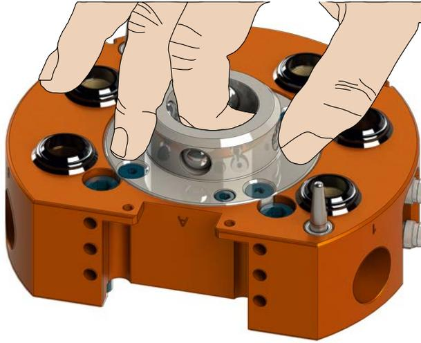
7. Apply a liberal coating of lubricant to the ball bearings, the male coupling (inside and out), and the alignment pins.
