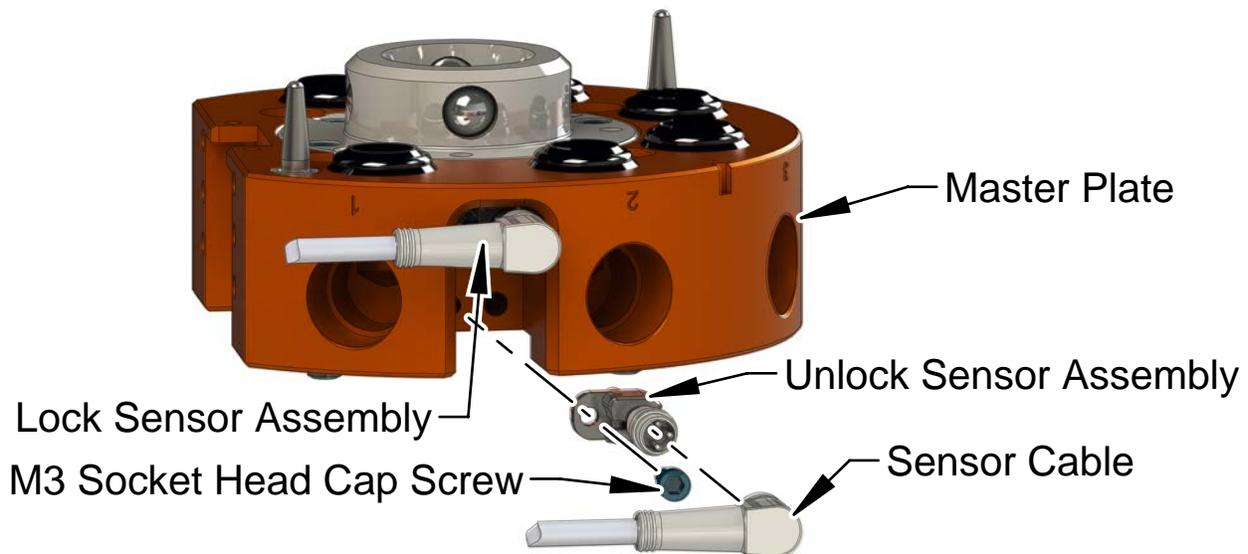
7. Insert the new lock and/or unlock sensor into the Tool Changer body as shown in [Figure 5.1](#). Make sure the O-ring is in place and seated properly on the back side of the sensor assembly.
