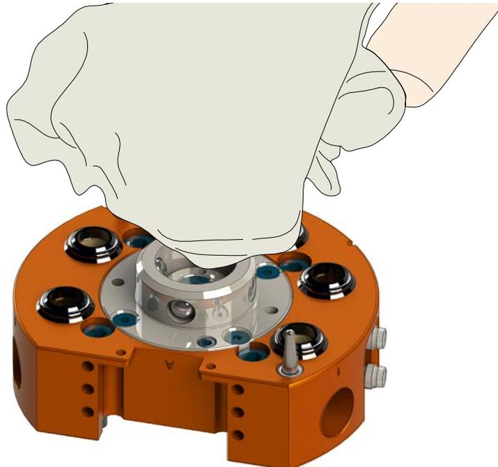
6. Check each ball bearing to make sure it moves freely in the male coupling. Additional cleaning may be necessary to free up any ball bearings that are sticking in place.
