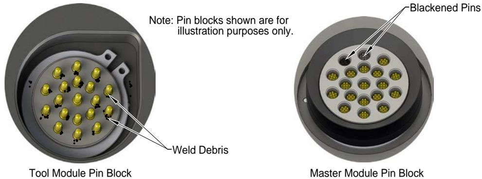
4. If debris or darkened pins exist, remove debris using a vacuum, and clean using a nylon brush (ATI Part Number 3690-0000064-60).
