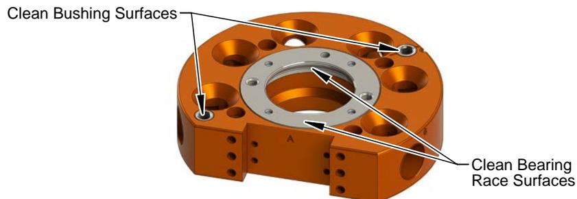
10. No application of lubrication is necessary on the Tool plate components.
