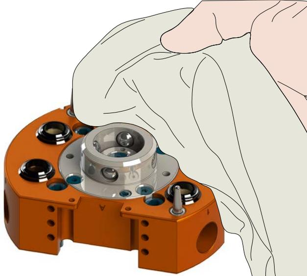
5. Use a clean rag to thoroughly remove any lubricant and debris from the inner surface of the male coupling and cam.
