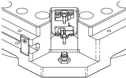
**Lock and Unlock Sensor Assemblies Replacement (Current Revision)**
