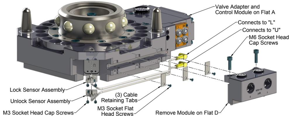
9. Route the new Lock and/or Unlock sensor cable into the cable channel of the Tool Changer body.
