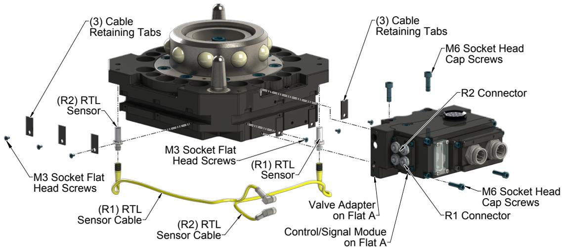
8. Install the sensor cable, routing the cable into the cable channel of the Tool Changer body.
