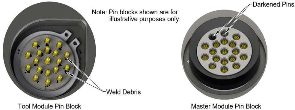
5. If debris or darkened pins are present, use a vacuum to remove the debris, and clean using a nylon brush (ATI Part Number 3690-0000064-60).
