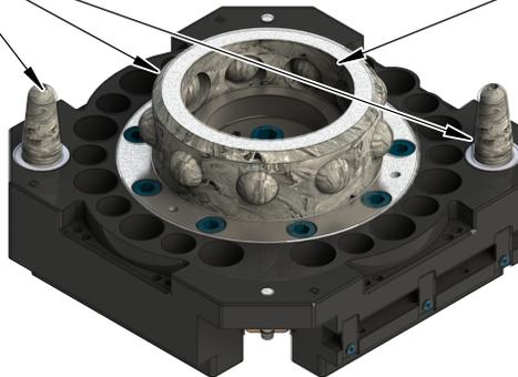
8. Use a clean rag to thoroughly remove any lubricant and debris from the Tool plate bearing race and bushings.
