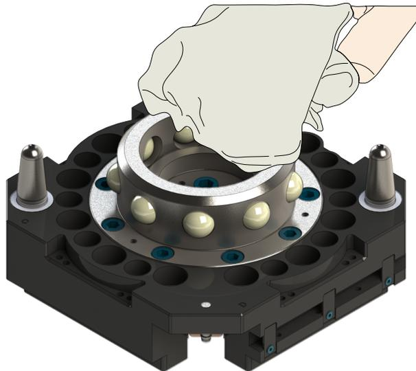
6. Check each ball bearing to make sure it moves freely in the male coupling. Additional cleaning may be necessary to free up any ball bearings that are sticking in place.
