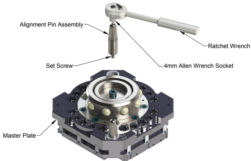
5. Alternately, use the access hole in the back side of the Master plate. If not already removed, remove the Master plate refer to [Section 2.3—Master Plate Removal](#).
