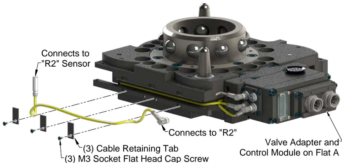
9. Install the sensor cable, routing the cable into the of the Tool Changer body.
