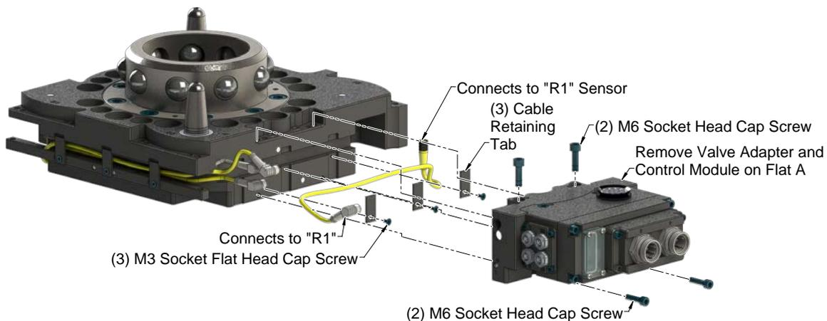
8. Install the sensor cable, routing the cable into the of the Tool Changer body.
