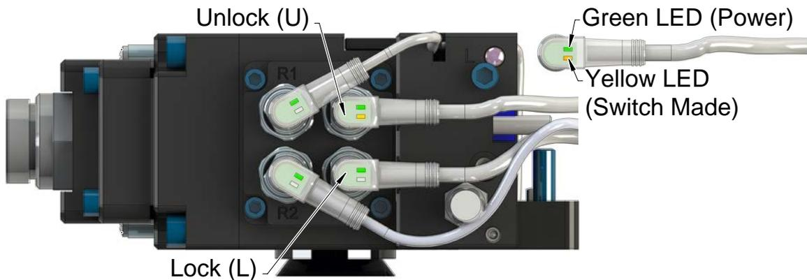
19. Confirm the operation of the Lock sensor by locking the Tool Changer and then checking to see if the Lock sensor cable LED is on.
