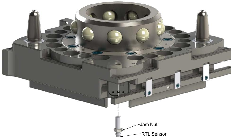
8. Screw the new RTL sensor into the Tool Changer body until the face of the sensor is flush with the surrounding face of the Master body.
