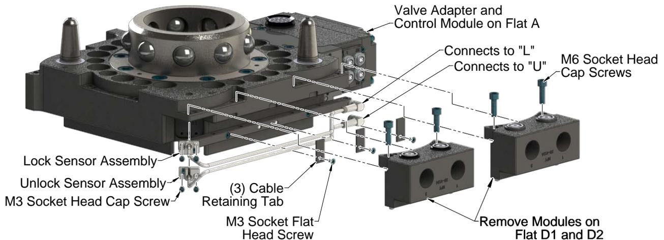
10. Install the new Lock and/or Unlock sensor assembly, routing the cable into the cable channel of the Tool Changer body.
