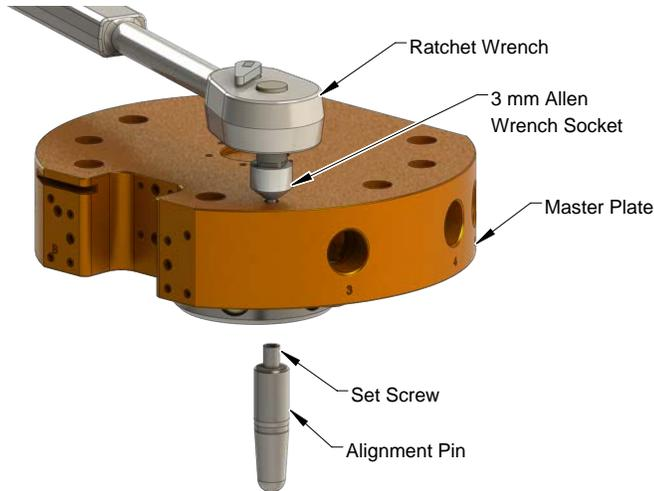
7. With the alignment been removed, verify that the assembly (pin and set screw) are intact. If the set screw portion of the assembly did not come out, remove it separately using the access hole in the back plate of the Master plate.
