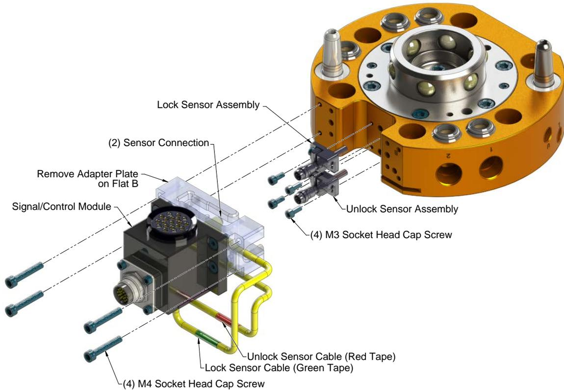
10. Install the new Lock and/or Unlock sensor.
