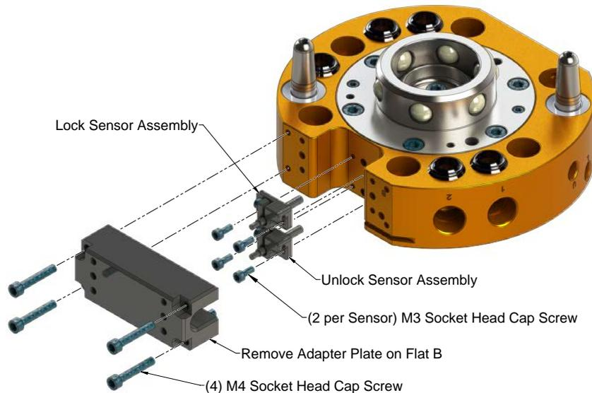
11. Install the new Lock and/or Unlock sensor.
