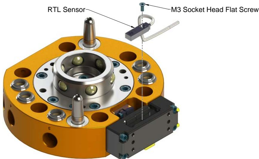
8. Feed the new sensor cable in between the adapter plate and the Tool plate.
