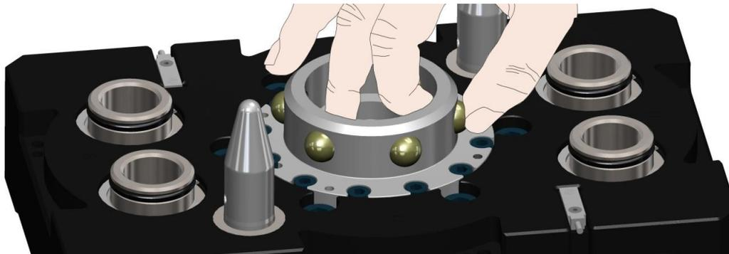
5. Apply a liberal coating of lubricant to the balls, the male coupling (inside and out), and the alignment pins.
