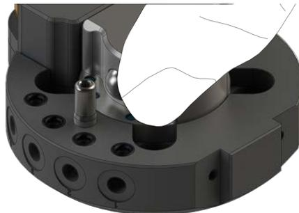
5. Apply a light coating of Superlube Multi-purpose Synthetic Grease with Syncolon, NSF (H1) Food Grade, NLGI 2 to the ball bearings, alignment pins, and O-rings.
