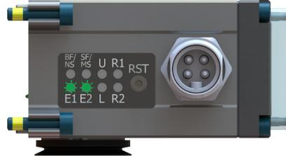
The Module Status (MS) LED is identified on the module as “MS”. It provides device status for power and proper operation. Refer to [Table 2.4](#) for an outline of this LED’s operation.
