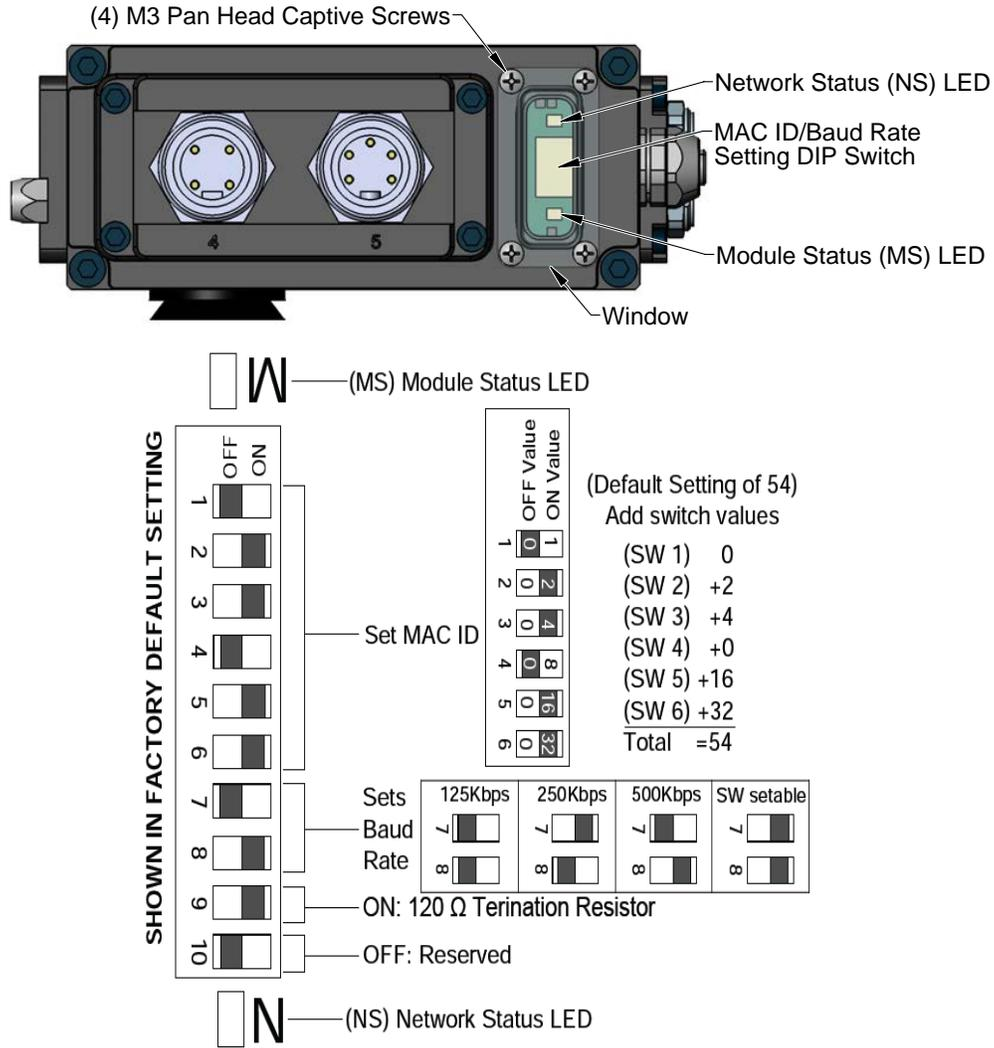
**NOTICE:** After adjustment is completed, ensure that the seal and window are re-positioned correctly to prevent a leakage path to inside the module.
