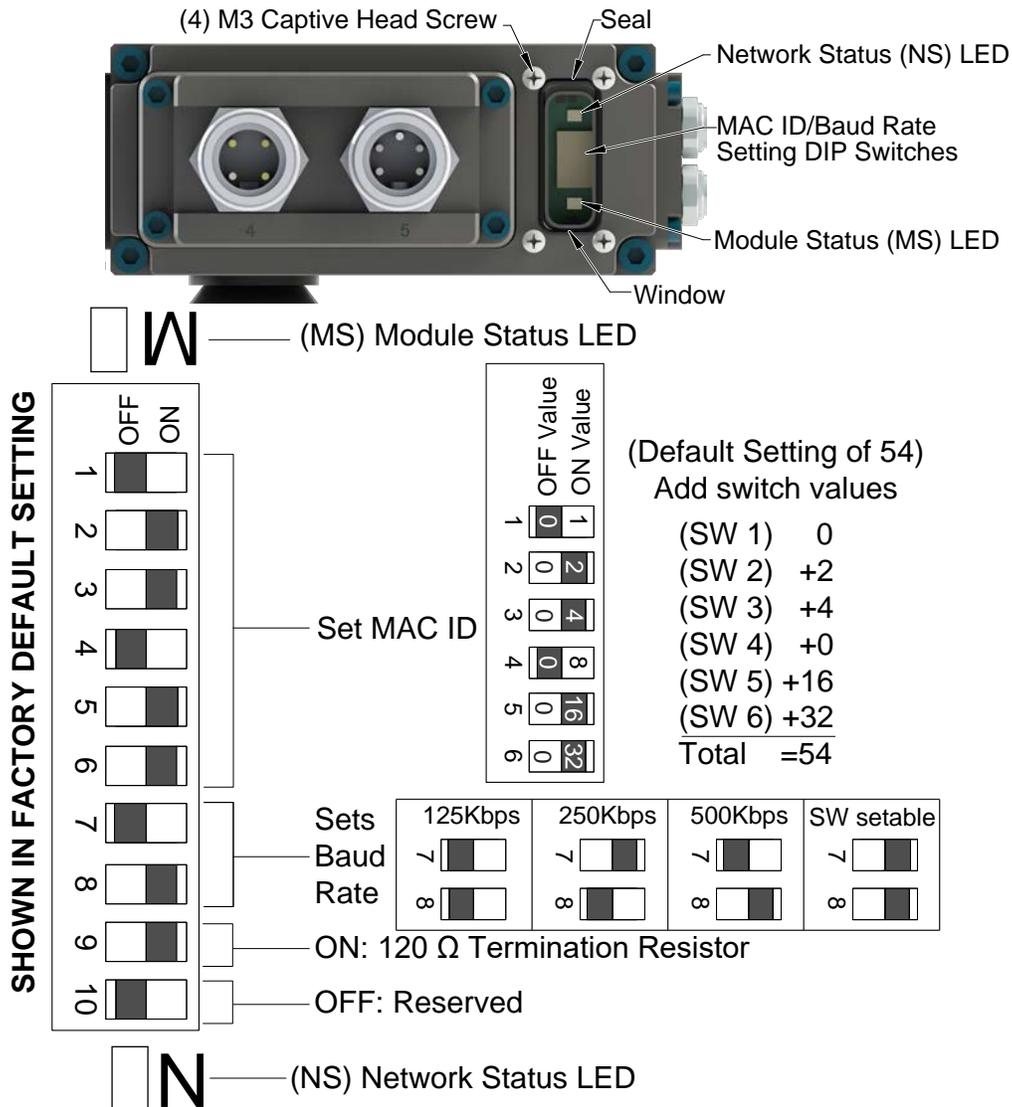
**NOTICE:** After adjustment is completed, ensure that the seal and window are re-positioned correctly to prevent a leakage path to inside the module.
