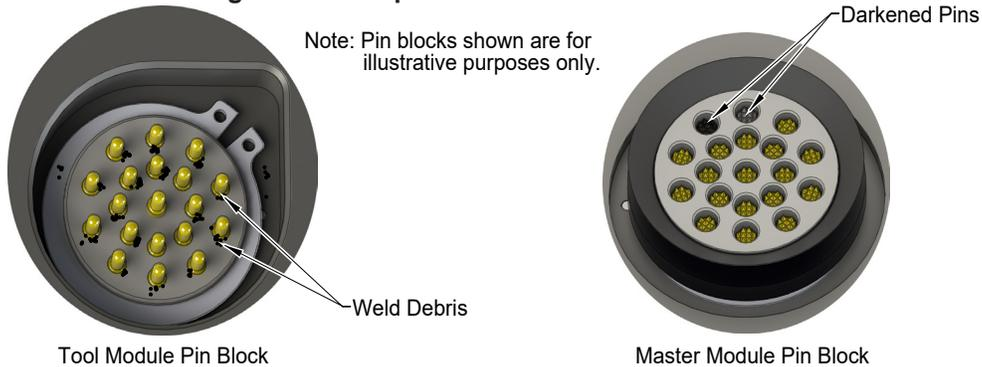
8. If debris or darkened pins exist, remove debris using a vacuum, and clean using a nylon brush (ATI Part Number 3690-0000064-60).
