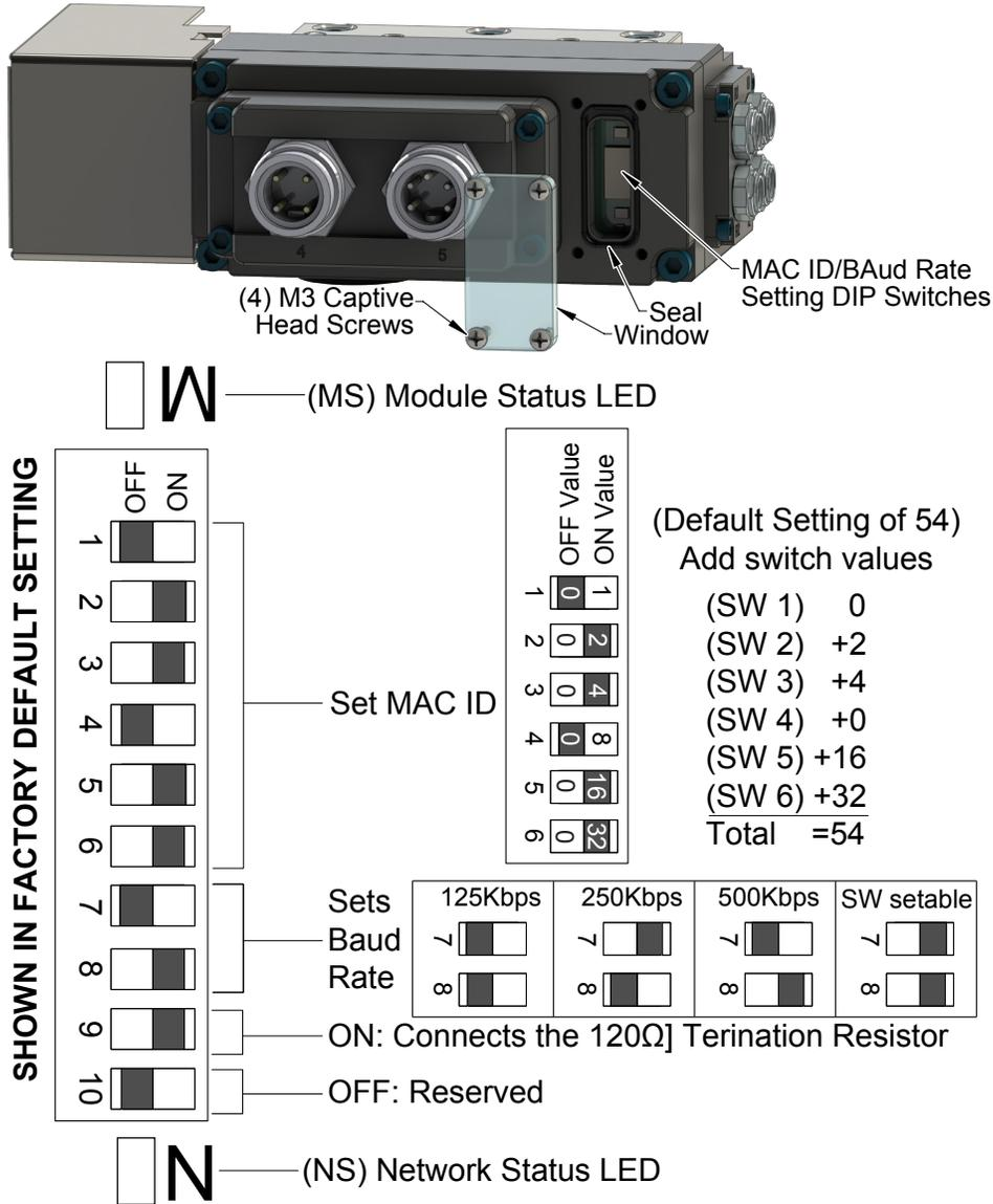
**NOTICE:** After adjustment is completed, ensure that the seal and window are re-positioned correctly to prevent a leakage path to inside the module.
