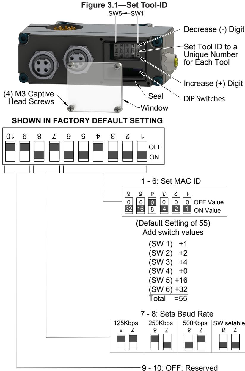
2. Use a non-conductive tool (e.g., plastic stylus) to press on the Tool-ID push buttons to increase (+) or decrease (-) the digit value. Set the Tool-ID to the desired unique digit number. Refer to [Section 9—Drawings](#) for Tool-ID output tables.
