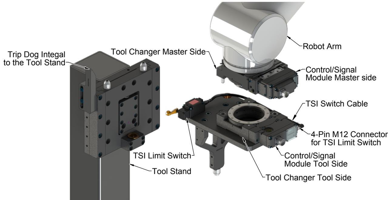
The DB15-M DB10-T modules rely on the status of the TSRV input to determine when it is appropriate to unlatch the Tool. The RTL sensors indicate if the Master and Tool are coupled while the TSRV input indicates when the TSI mechanical switch on the Tool is actuated, thereby indicating that the Tool is in the stand.
