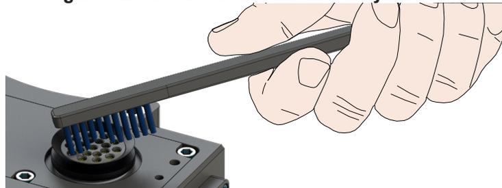
9. Inspect the Master and Tool pin blocks for stuck pins or severe pin block damage.
