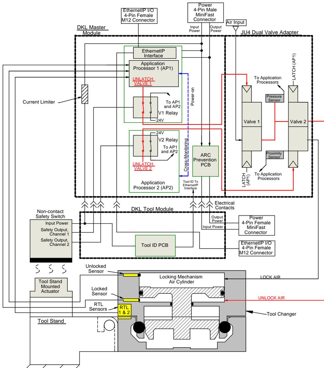
The safety switch (not included with module) is connected to the Tool side module and the actuator is mounted to the tool stand. The safety switch is connected to the Tool module by a five conductor M12 cable. Refer to the Dual Double Solenoid Valve Adapter Manual (9620-20-C-Jxx Valve Adapters with Dual Double Solenoid, Valve Pass-through, Proximity and Pressure Sensors) for detailed information on the dual double solenoid valve functionality.
