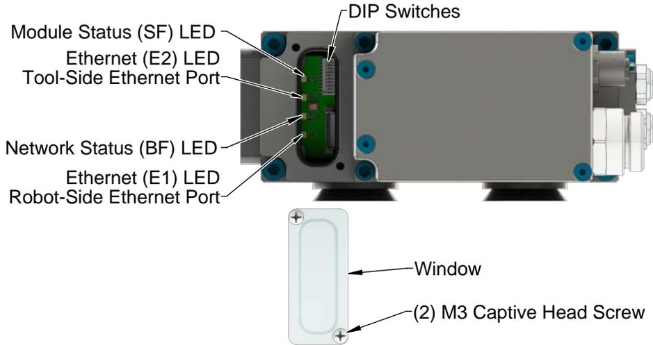
**Figure 2.12—EtherNET/IP Master Module DIP Switch Settings**
