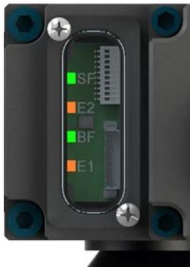
Module Status (SF) status LED is identified on the module as “SF”. It provides device status for power and proper operation. Refer to *Table 2.3* for an outline of this LED’s operation.
