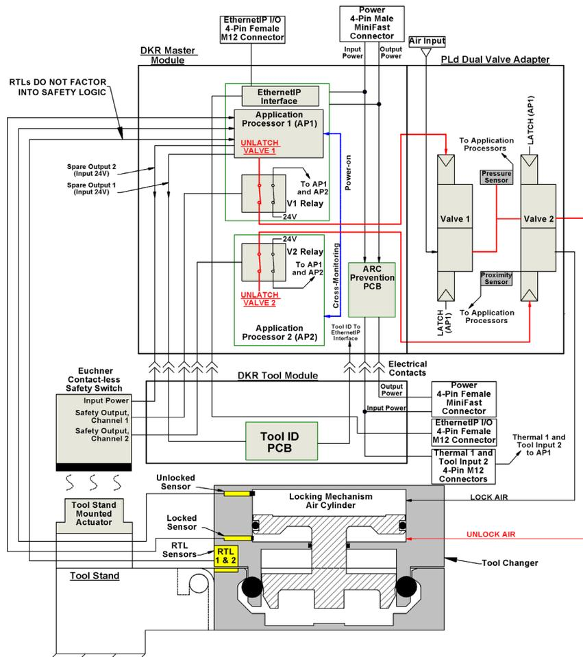
The safety switch (not included with module) is connected to the DKR Tool side module and the actuator is mounted to the tool stand. The safety switch is connected to the DKR Tool module by a (5) conductor M12 cable.
