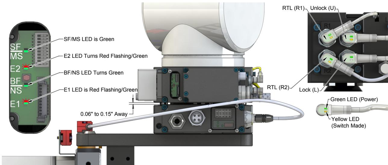
2. Robot and Master move into the Tool, are parallel and within 0.06" to 0.15" of the Tool (for example: the module electrical contact pins are touching but the Ready-to-Lock sensors have not yet sensed the targets on the Tool).
