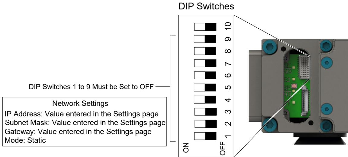
Connect to the Integrated Web Server on the DKR Master Module using a laptop and open the Settings page. Refer to [Section 2.2—Integrated Web Server](#):
