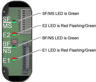
Module Status (SF/MS) status LED provides device status for power and proper operation. Refer to *Table 2.3*. Network Status (BF/NS) status LED provides Ethernet/IP status information. Refer to *Table 2.4*.
