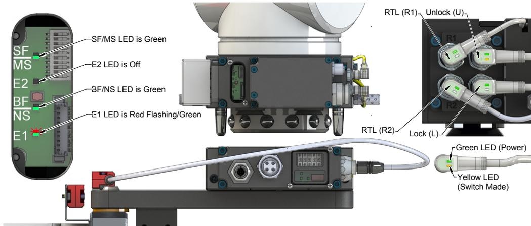
1. The robot and Tool Changer Master are free of the stand or storage location, the Tool Changer is uncoupled and the Tool Changer locking mechanism is fully retracted (unlocked condition). The Tool is by itself in the tool stand. No error or fault conditions exist.
