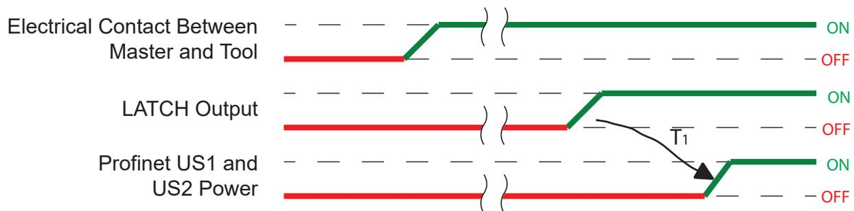
$T_1$  = Power Switch ON-delay (Less than 100 ms)
