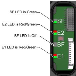
The System Failure (SF) status LED is identified on the module as “SF”. It provides device status for power and proper operation. Refer to [Table 2.4](#) for an outline of this LED’s operation.
