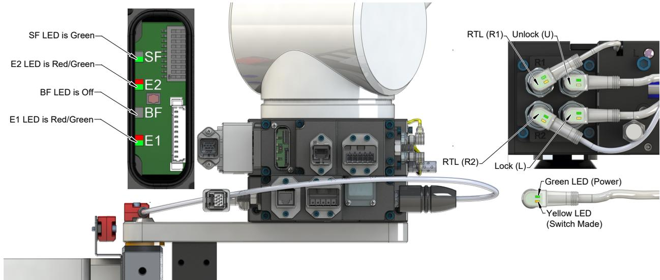
7. Robot moves into the Tool stand with the Tool Changer coupled. **Everything is OK** bit is ON.
