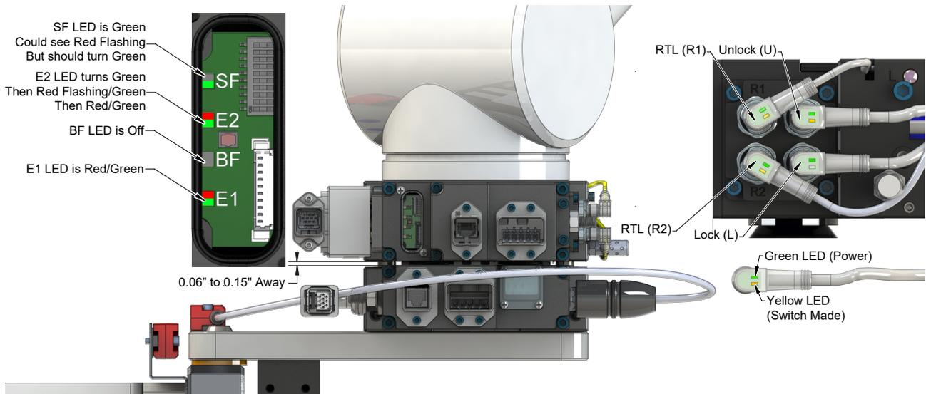
3. Robot and Master move within 0.06” of the Tool and safety switch is within range.
