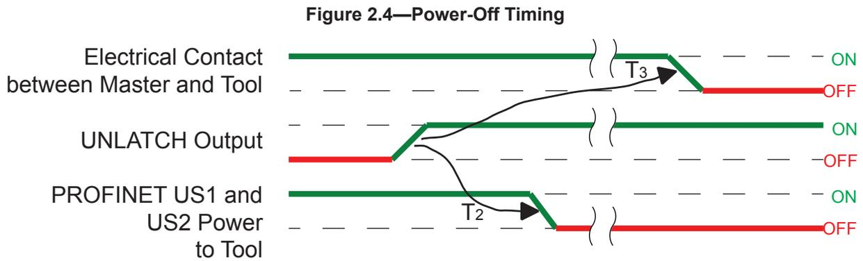
$T_2$  = Power Switch OFF-delay
