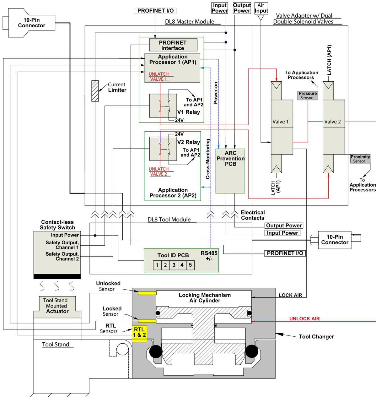
A second set of contacts on the V1 and V2 relays also provide diagnostics to the Application Processors. A dual double solenoid valve adapter is equipped with two double solenoid valves. Pressure and proximity sensor outputs provided by the valve adapter are evaluated by the Application Processors for diagnostic purposes.
