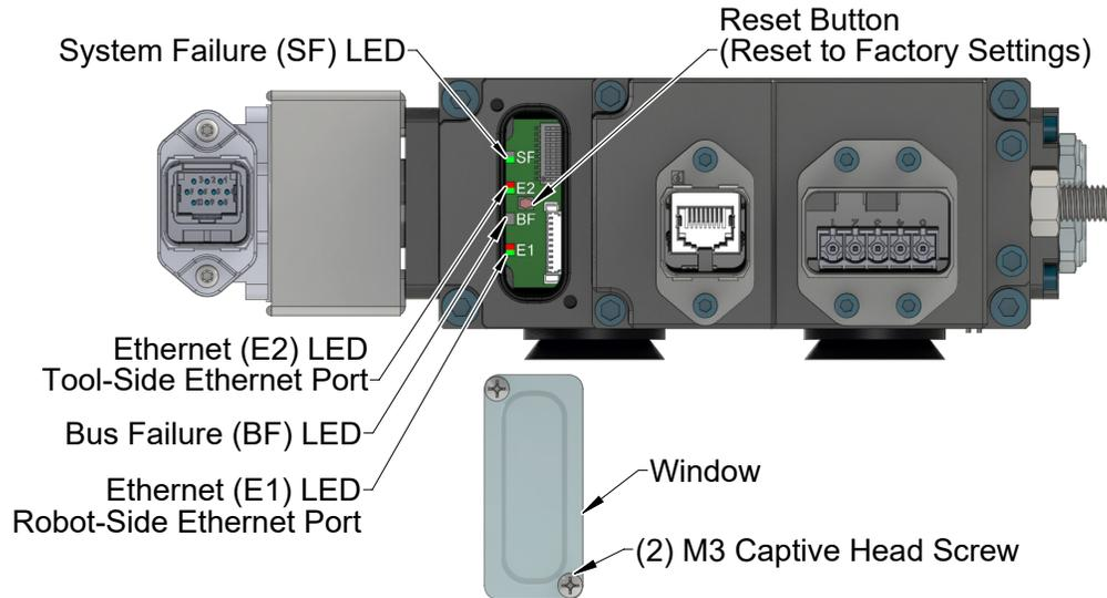
11. Re-install the window and tighten the (2) M3 pan head captive screws.
