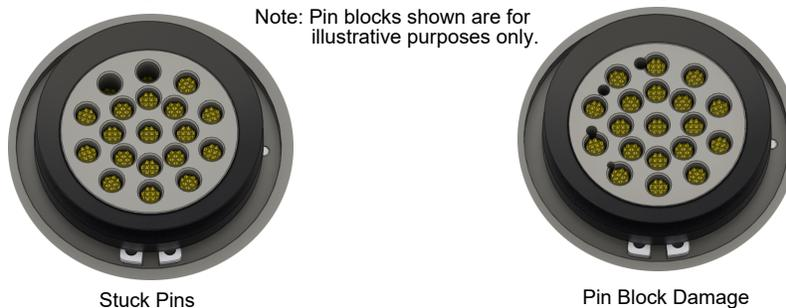
7. If pins become stuck or if there is damage to the pin block, contact ATI for either a possible pin replacement procedure or module replacement.
