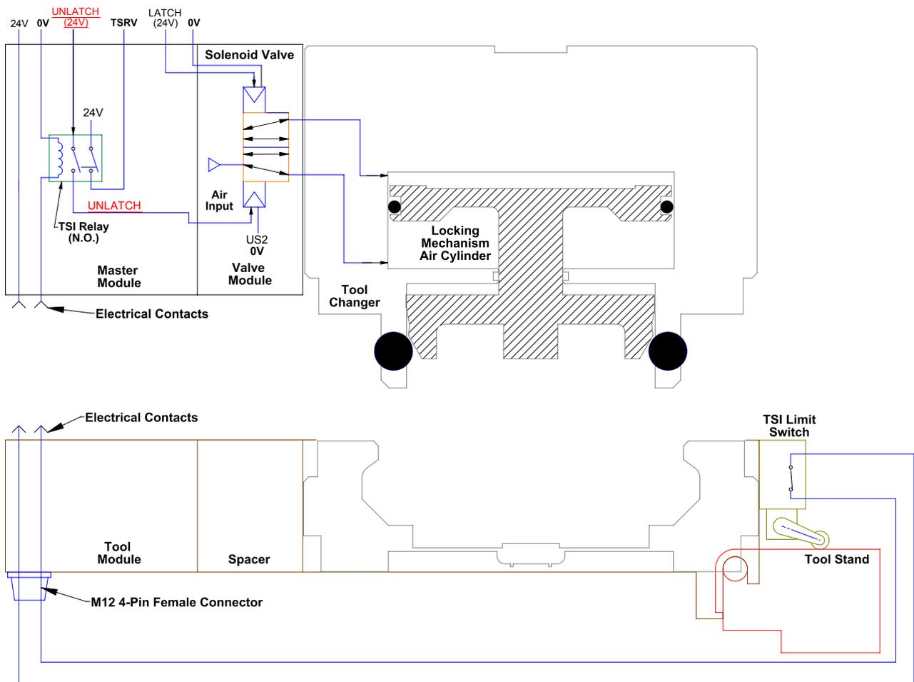
The Master and Tool are within coupling distance and the electrical contacts meet. The TSI relay closes because the TSI limit switch is actuated and the electrical contacts meet. It is now possible for the TSI relay to pass the unlatch signal from the robot to the solenoid valve.
