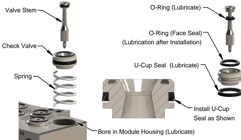
18. Install the valve stem. The check valve piston must be pushed down flush with the mating surface of the Master housing in order to install the threaded end of the valve stem. Do not damage the U-cup seal around the check valve piston. A small, flat-head screwdriver can be used to ensure that the U-cup seal is fully located in the recess and not folded over itself prior to screwing in the valve stem. Tighten the stem to 10 in-lbs (1.1 Nm).
