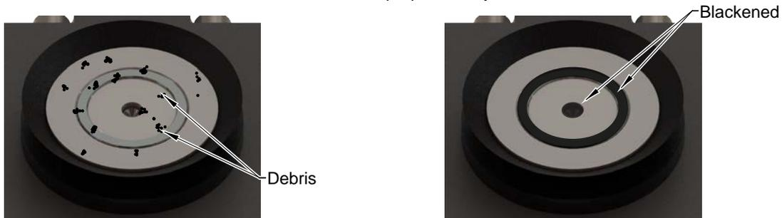
5. If debris or blackened center pin and shielding ring are present, use a vacuum to remove the debris, and clean using a nylon brush (ATI Part Number 3690-0000064-60).
