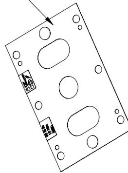
9005-20-1895 Insulator Sheet. Used between fiberglass cover and aluminum plate.
