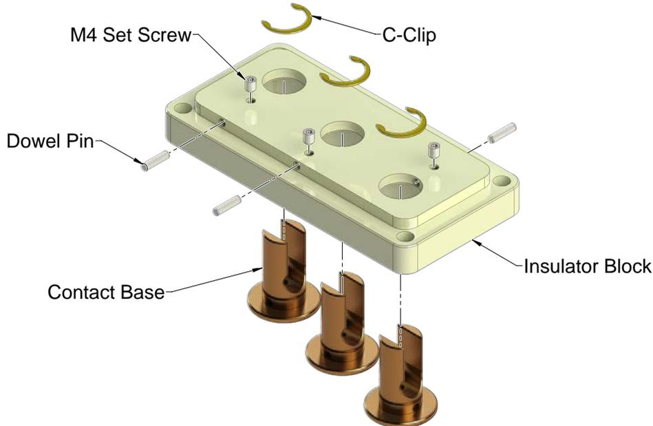
15. Install the new contact base into the insulator block in the correct orientation. Refer to [Figure 5.4](#).
