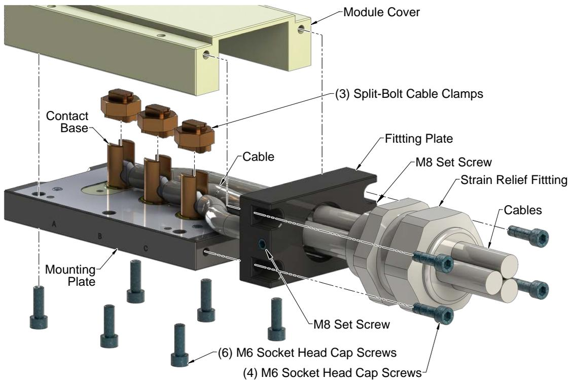
9. Insert each prepared cable end into the appropriate contact base and replace the split-bolt nut. Make sure that no loose wire filaments are protruding from the contact bases. Also, ensure that the clamping lugs are not clamped on the cable insulation and the entire clamp lug is contacting the copper wire. Tighten to 90 in-lbs (10 Nm) using a 13/16 wrench.
