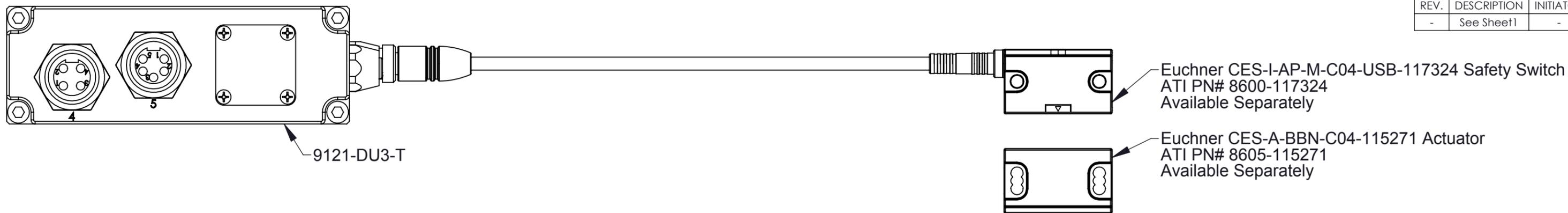
**Figure 1: Connection of 1X Euchner CES-AP-C01 Safety Sensor**
