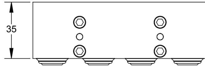
4X G 3/8 (BSPP) Pass-Thru Ports (Air/Vacuum Service)
