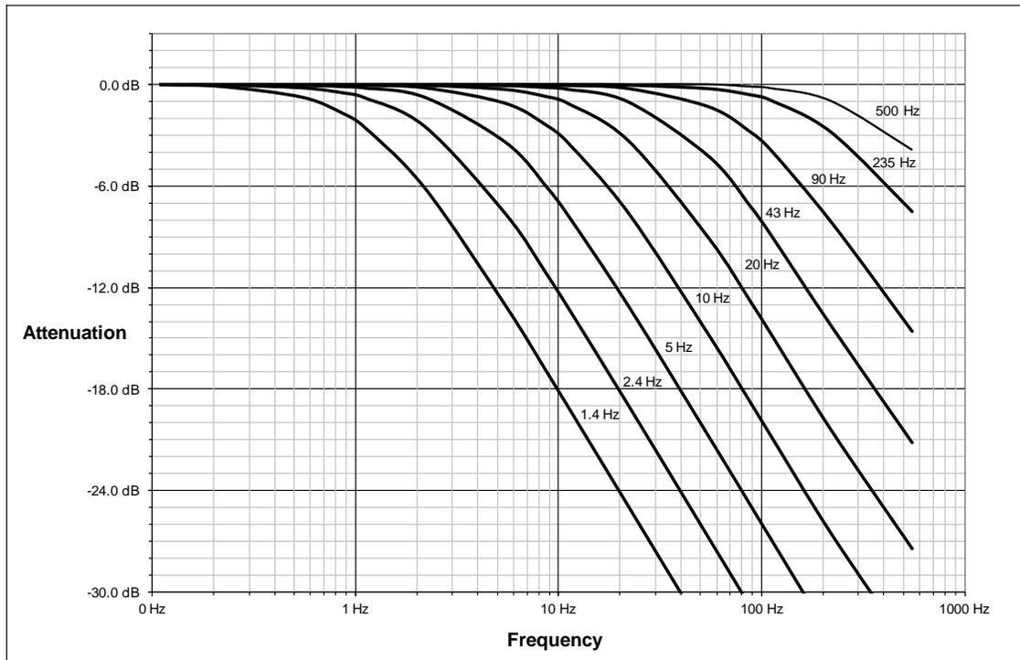
Figure 4.5—Filter Attenuation at 4 kHz Sample Rate
