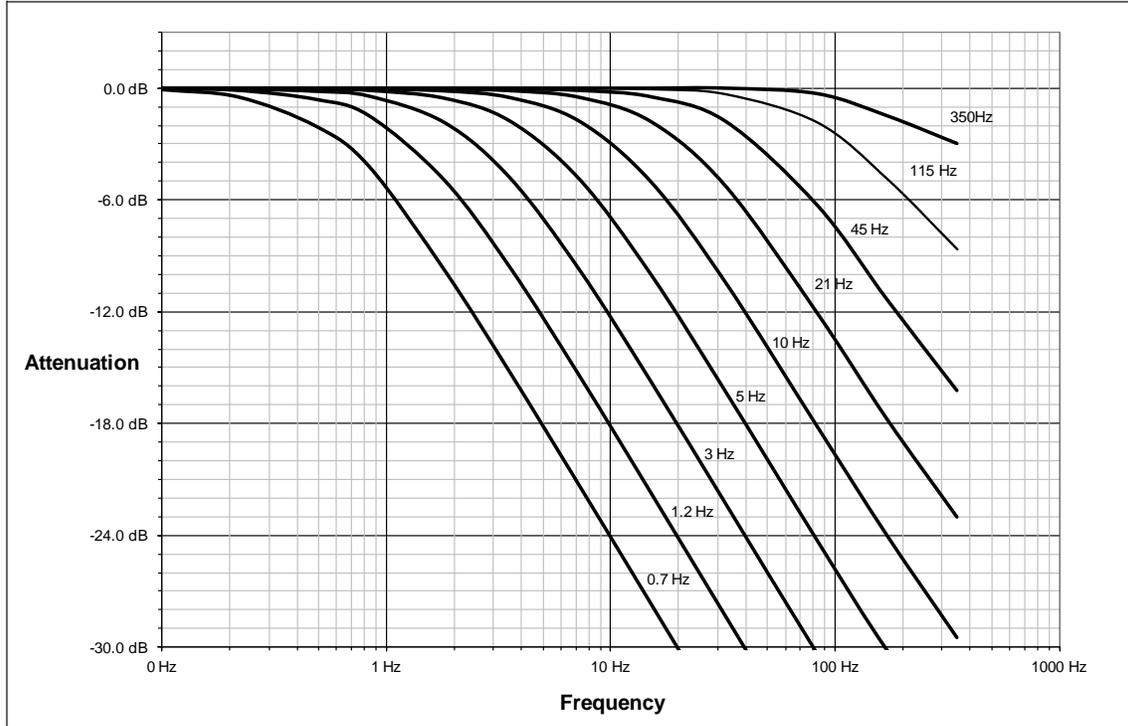
Figure 4.4—Filter Attenuation at 2 kHz Sample Rate
