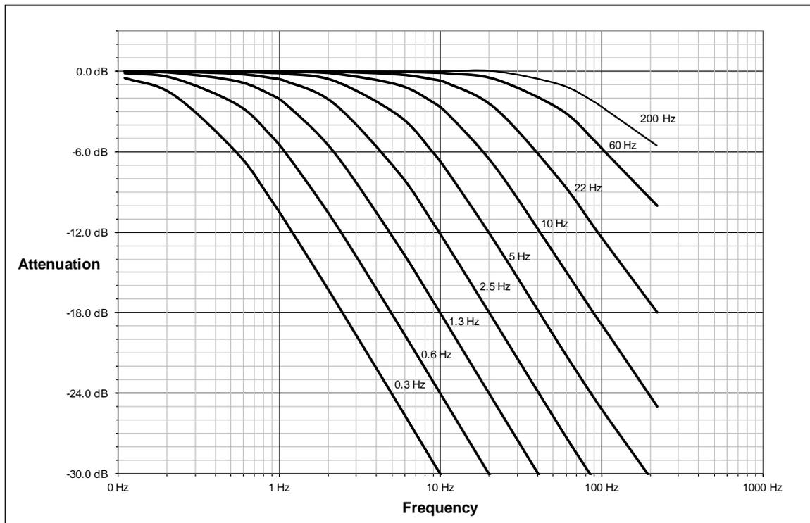
Figure 4.3—Filter Attenuation at 1 kHz Sample Rate
