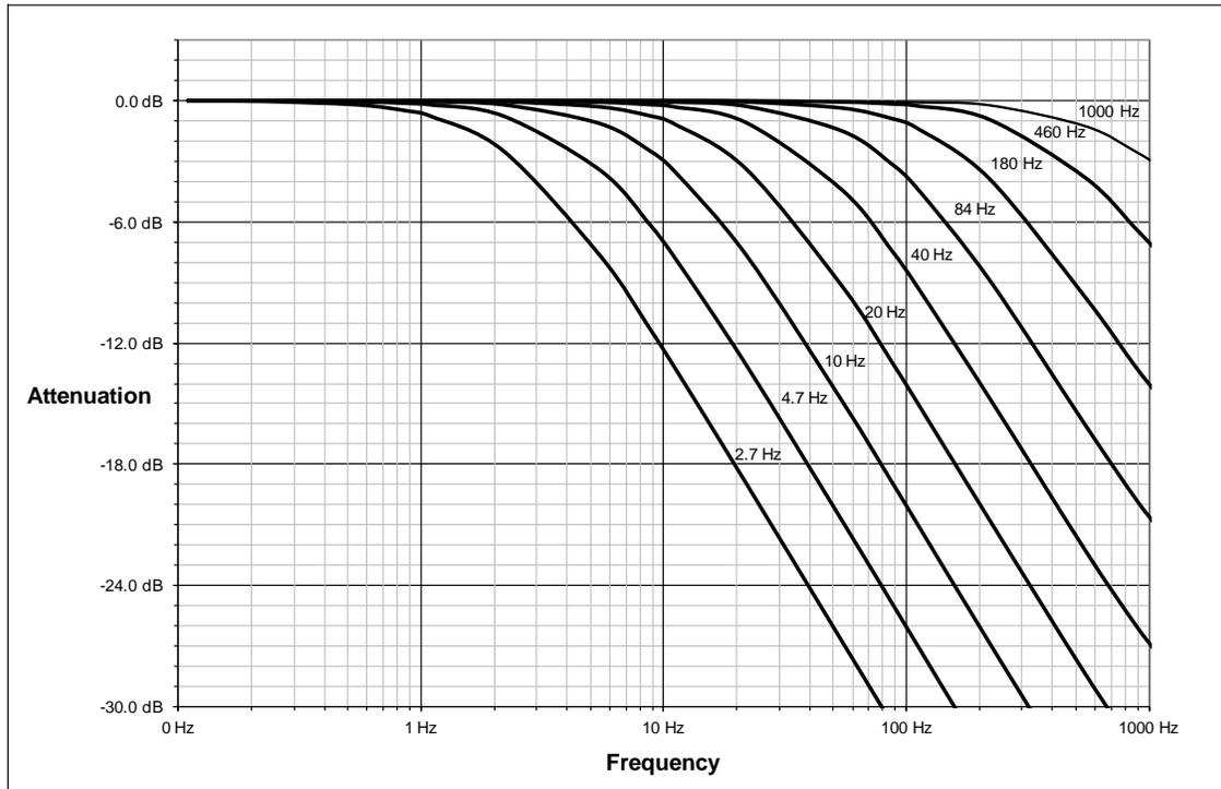
Figure 4.6—Filter Attenuation at 8 kHz Sample Rate
