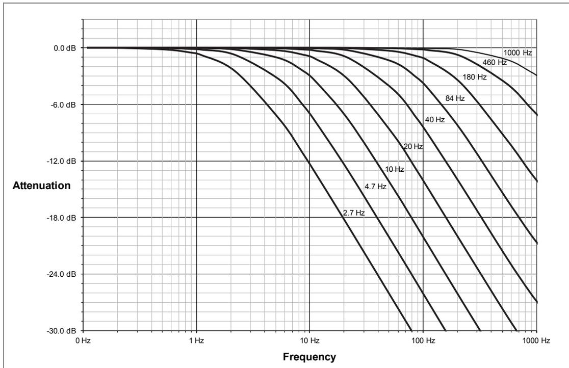
Figure 5.6—Filter Attenuation at 8 kHz Sample Rate
