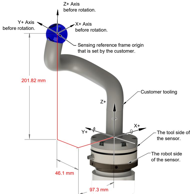
After the displacements, the user point of origin rotates in the following order:
