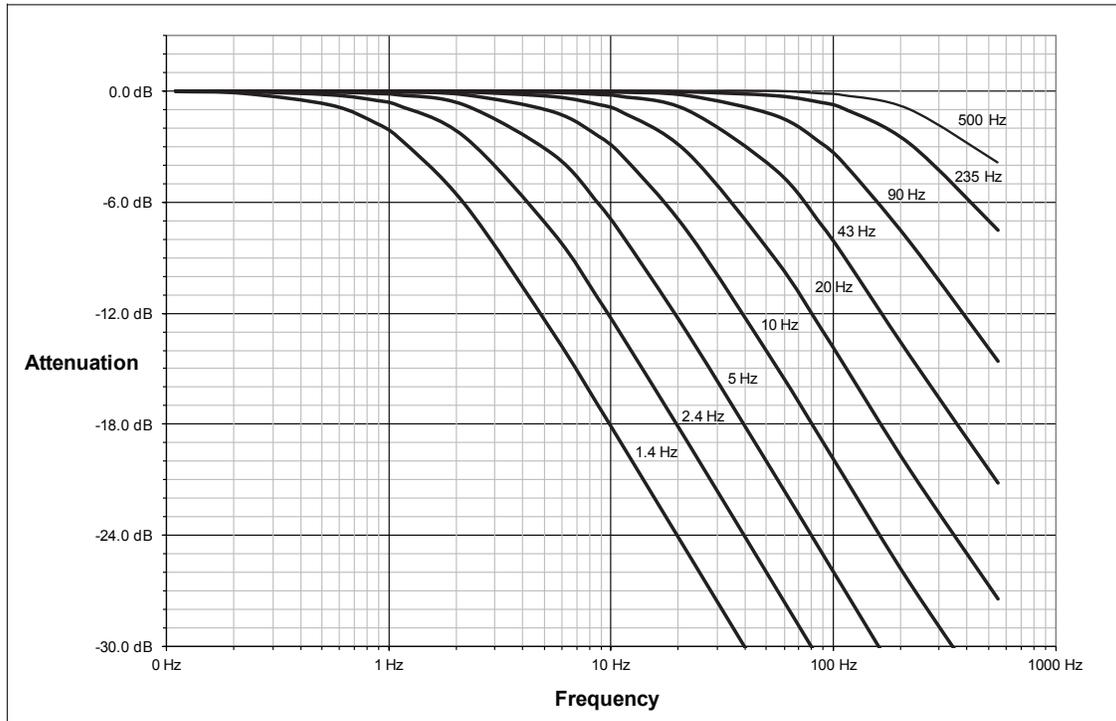
**Figure 5.5—Filter Attenuation at 4 kHz Sample Rate**
