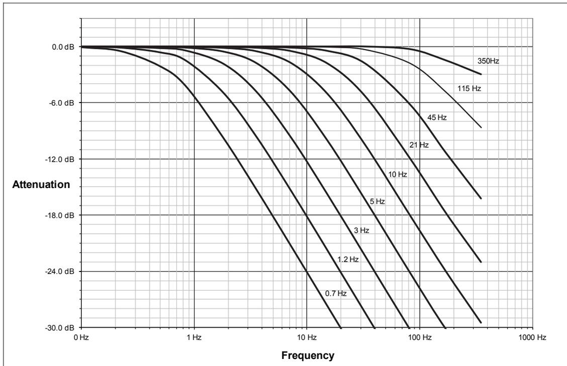
**Figure 5.4—Filter Attenuation at 2 kHz Sample Rate**
