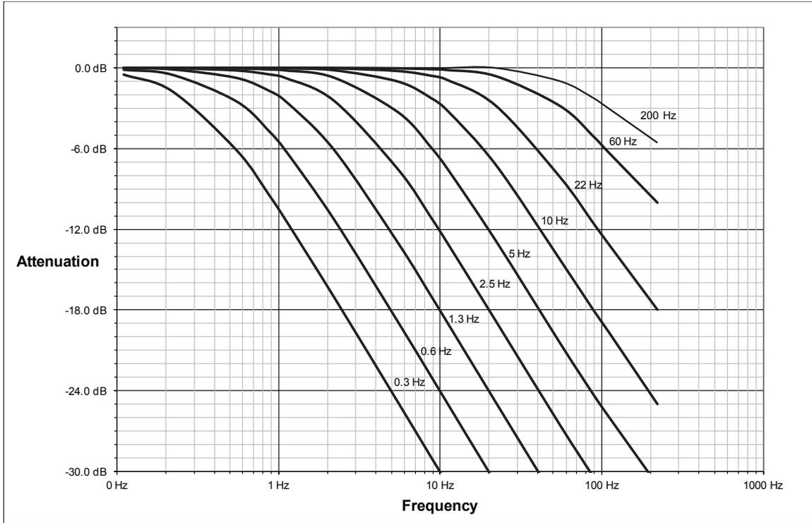
Figure 5.3—Filter Attenuation at 1 kHz Sample Rate
