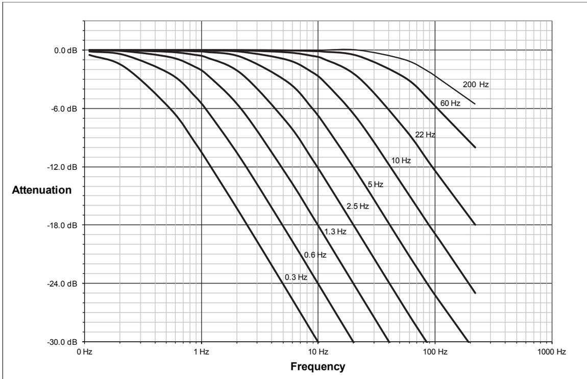
Figure 4.4—Filter Attenuation at 1 kHz Sample Rate
