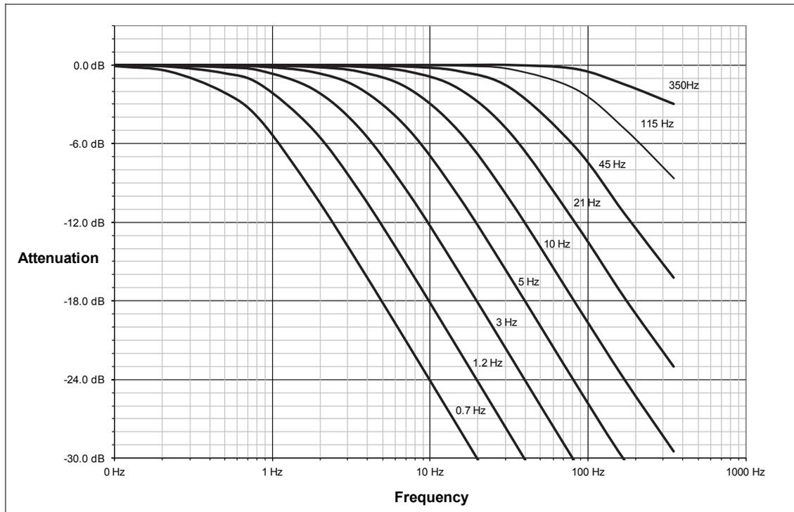
**Figure 4.5—Filter Attenuation at 2 kHz Sample Rate**
