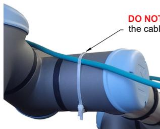
**DO NOT USE** zip ties to restrain the cable around the robot arm.
