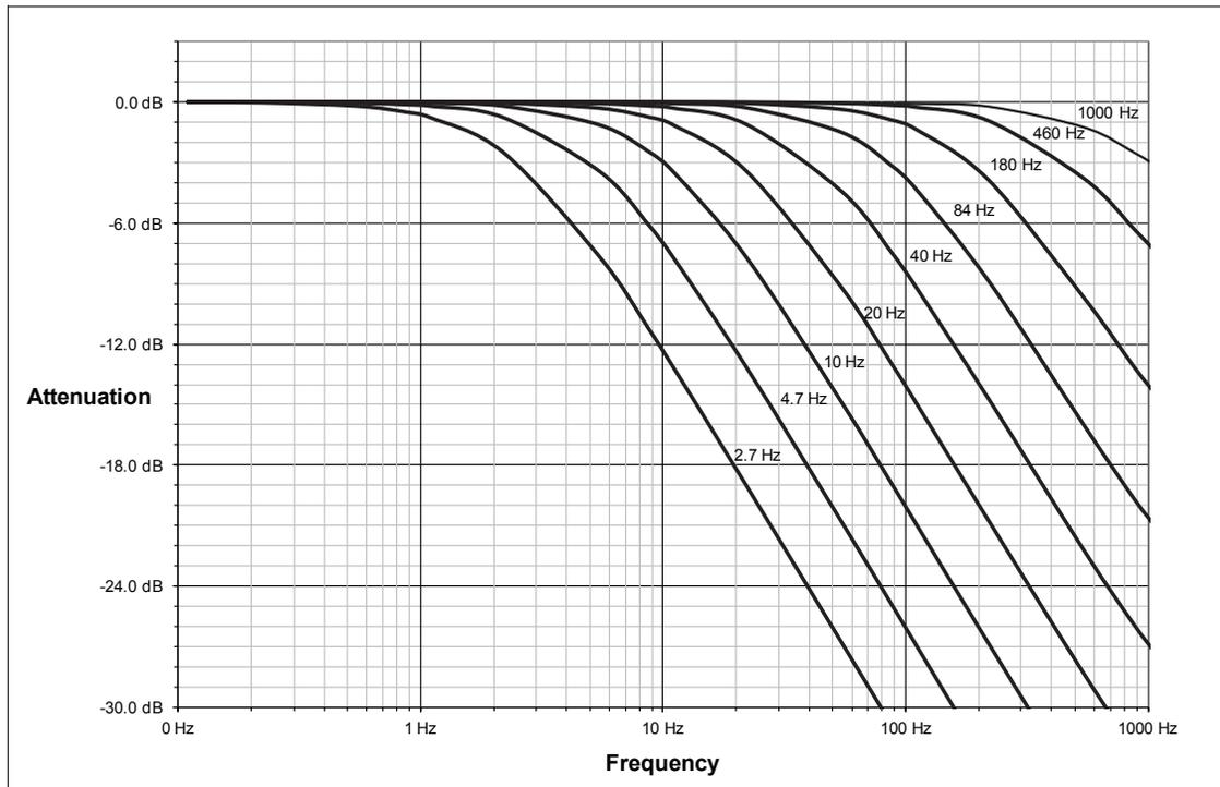
Figure 4.7—Filter Attenuation at 8 kHz Sample Rate
