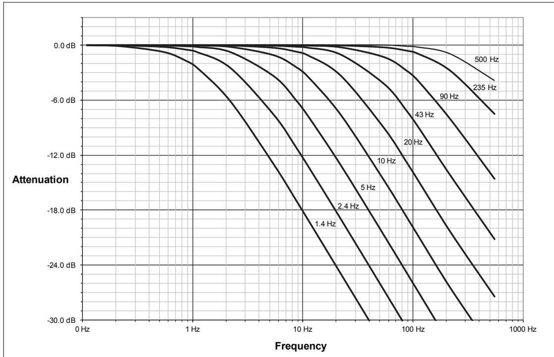
**Figure 4.6—Filter Attenuation at 4 kHz Sample Rate**
