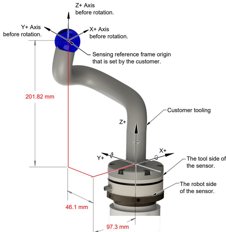
After the displacements, the user point of origin rotates in the following order:
