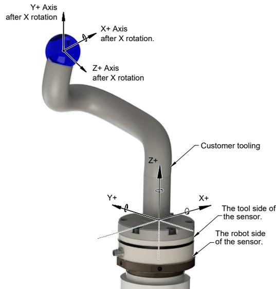
2. The second rotation is about the Y-axis of the new user output reference frame.
