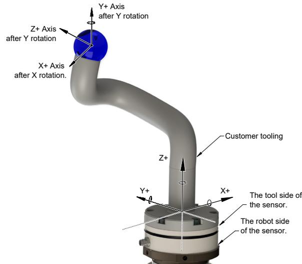
3. The third and final rotation is about the Z-axis of the new user output reference frame.
