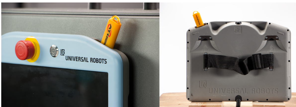
Figure 4.1—Insert USB Drive into USB Port on the Teach Pendant
