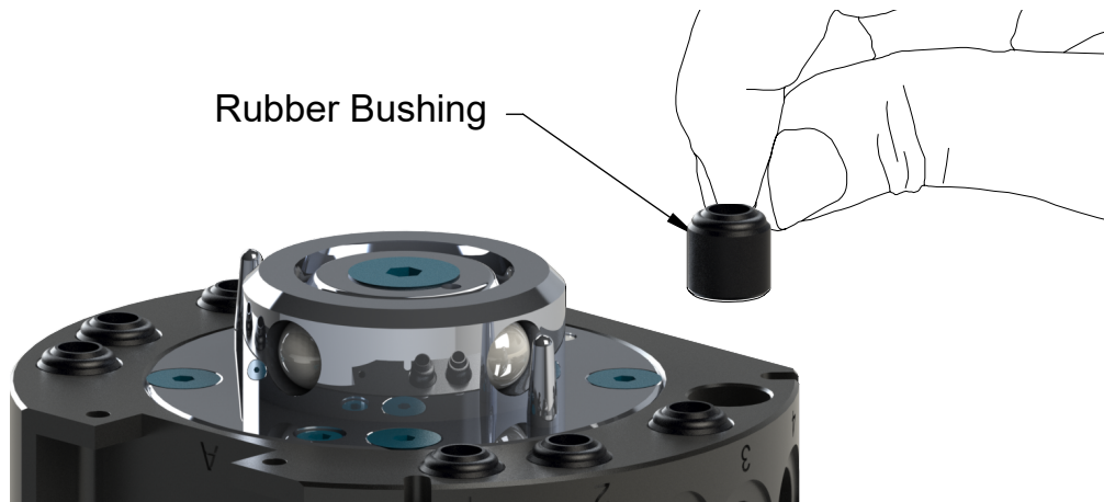
Figure 6.5 —Rubber Bushing Replacement
