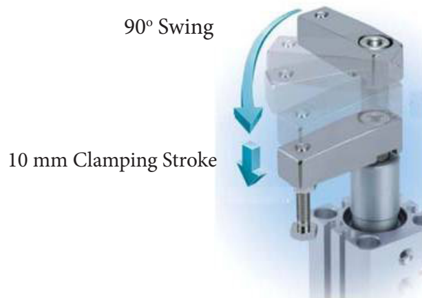
Figure 2.2—Adjustable Actuator Arm Swing and Stroke
