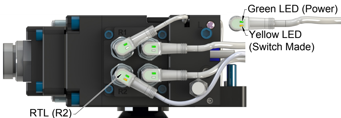
Figure 5.11—RTL (R2) Sensor Cable LEDs
